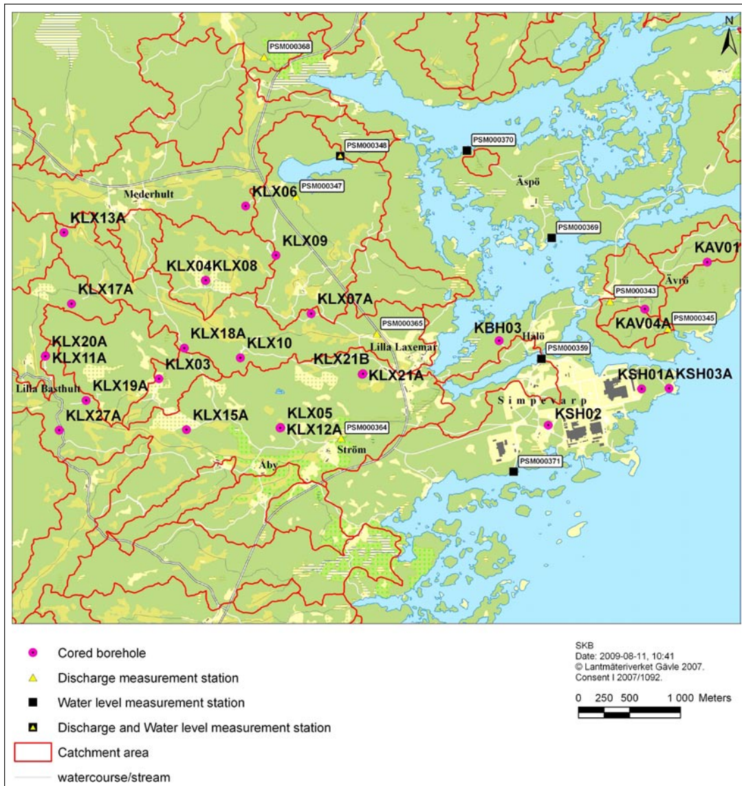
Figure 3-3. Map of the percussion drilled parts of the deep cored boreholes (ie the telescopic sections) during the site investigation in Oskarshamn, subareas Simpevarp (KSH, KAV and KBH holes) and Laxemar (KLX holes). Also shown on the map are drainage areas and surface water discharge stations.
