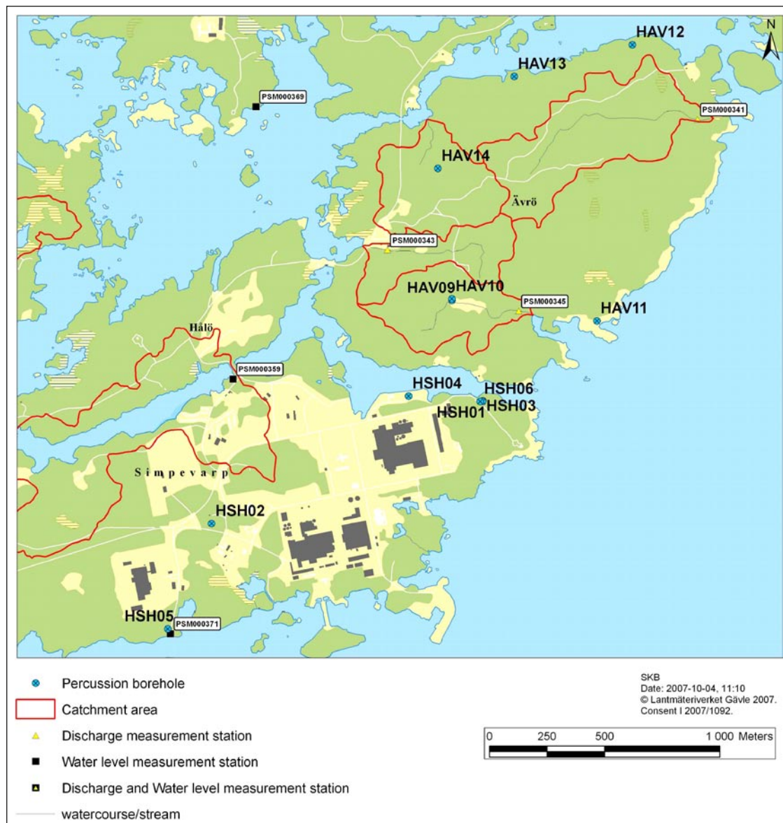
Figure 3-1. Map with percussion boreholes in the Simpevarp subarea together with drainage areas and surface water discharge measurement stations.
