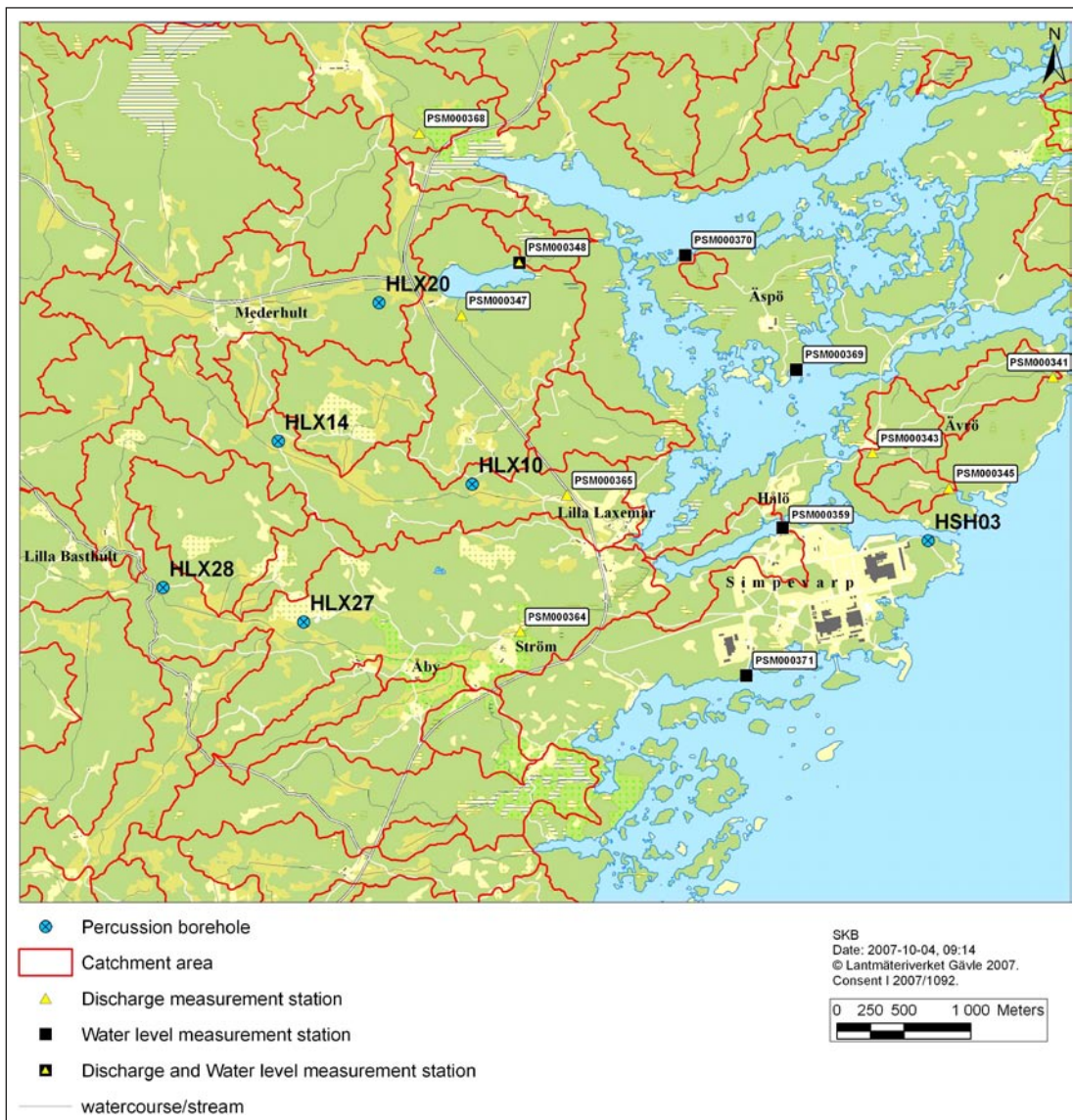
Figure 3-6. Map of flushing water wells in the Oskarshamn site investigation area together with catchment areas and surface water level and discharge measuring stations.
