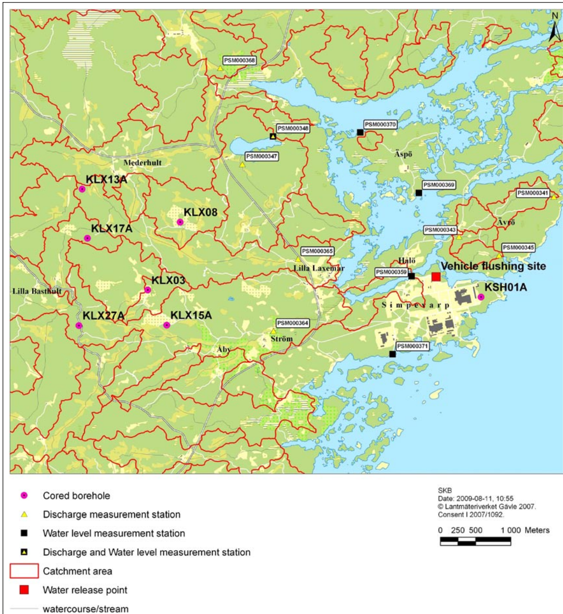
Figure 3-8. Map of boreholes where complete chemical characterization has been done or is planned to be performed (KSH01A, KLX03, KLX08, KLX13A, KLX17A, KLX15A and KLX27A). The main water emissions have arisen not from the actual sampling but from rinse pumping in between sampling events in KLX03 and KLX08.
