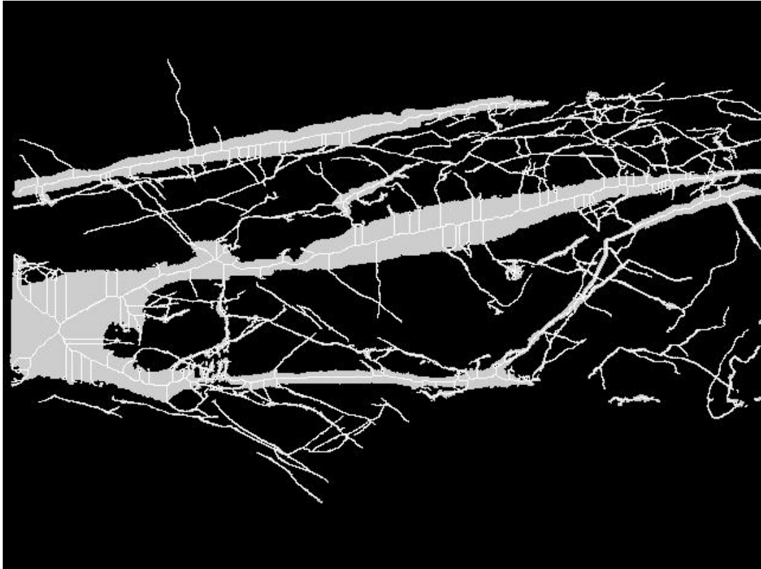
Figure 6-10. B2-a1, Network image overlay on the binary image; here, the grey colour represents the detected fractures, and the white colour represents the skeletons.
