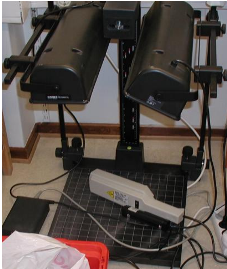
Figure 2-11. Image acquisition device: A box (red filled with fine sand; two ordinary lamps, the position of which can be adjusted; a plate with scales for samples and an ultraviolet (UV) lamp (grey with handle).
