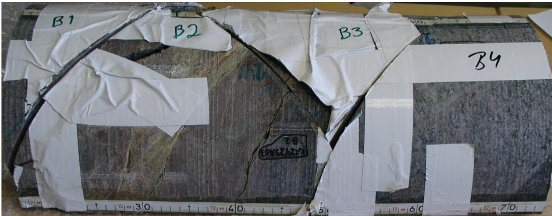
Figure 2-2. The core was cut along the core axis into two halves. Only one half (upper half) was used in the current study. This image shows samples B1, B2, B3 and B4 from borehole KA2423A03. The left side of the core is positioned closest to the tunnel and the intersection with the fracture zone centre is at 2.4 m borehole depth /Maersk-Hansen and Staub 2004/. (N.B. the reference tapes that can be observed in some photographs do not refer to borehole depth and were used only for relative measurements.)
