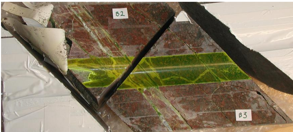
Figure 2-3. This figure is similar to Figure 2-2, but the samples (B2 and B3 from borehole KA2423A03) are rotated such that the cut surfaces are seen. The trace of the 76 mm injection hole may be noted in the centre of the photograph (light green epoxy). (Up direction is inwards the image.)
