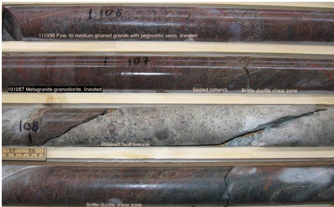
Figure 5-7. Character of deformation in the interval ~107–110 m borehole length, KFR101. Lineated fine- to medium-grained granite at ~106 m, lineated metagranite-granodiorite at ~107 m. Brittle-ductile shear zone at ~107.30–110 m with a core consisting of a polymict fault breccia and minor crush.
