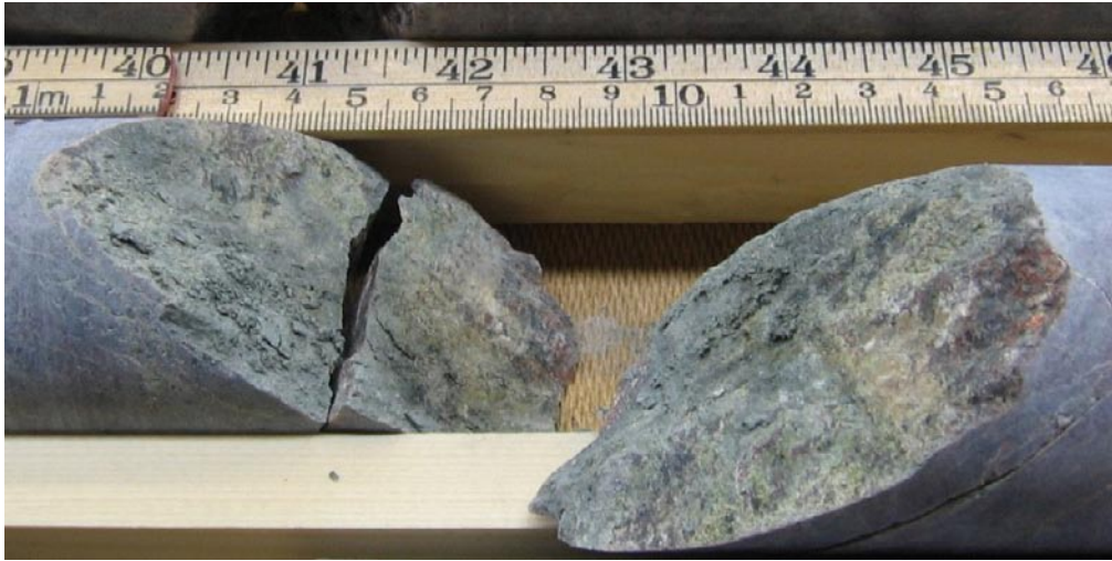
Figure 5-4. Clay-filled open fracture at 103.03 m borehole length in KFR101.
