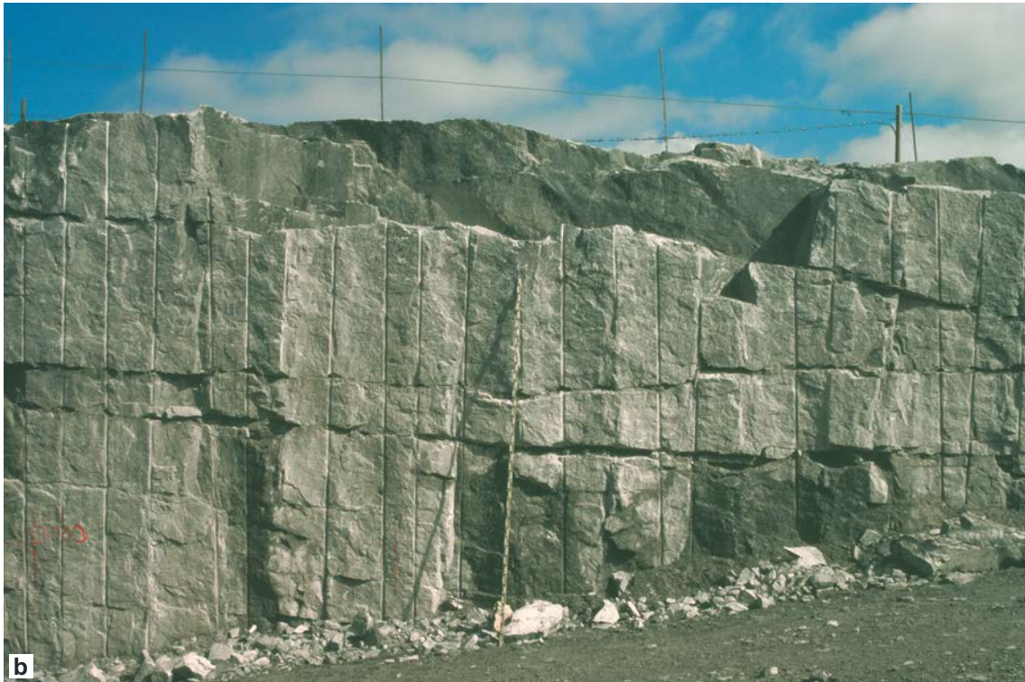
Figure 2-3. A: Cross-section illustration of the uppermost part of the bedrock. P = precipitation, E = evapotranspiration, R = Runoff (from /SKB 2008a/). B: Observed horizontal fractures in constructing the cooling water canal to the Forsmark nuclear power plant (from /Carlsson and Christiansson 2007/).
