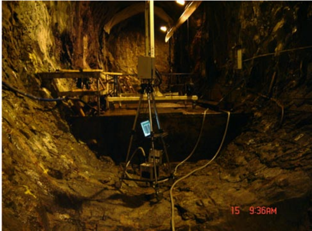
Figure 7-3. Field scanning in the TASQ tunnel at ÄSPÖ.
