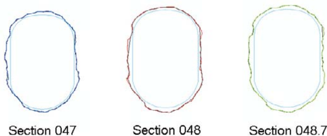
Figure 7-11. Planned and as-built geometry in the shady area. Compare group a) in Figure 9-22.
