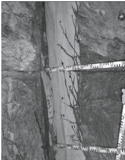
Figure 3-5. An example of the measurements of fractures in the cut-out at section 47. Reproduced from /Olsson et al. 2004/.
