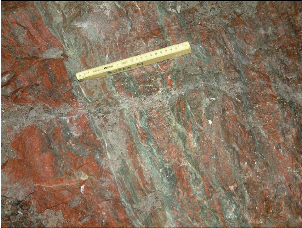
Figure 4-2. Close up photo of a local part of the shear zone running along TASQ. The strong foliation in the zone can be seen aligned with minor fractures filled with calcite /Magnor 2004/.
