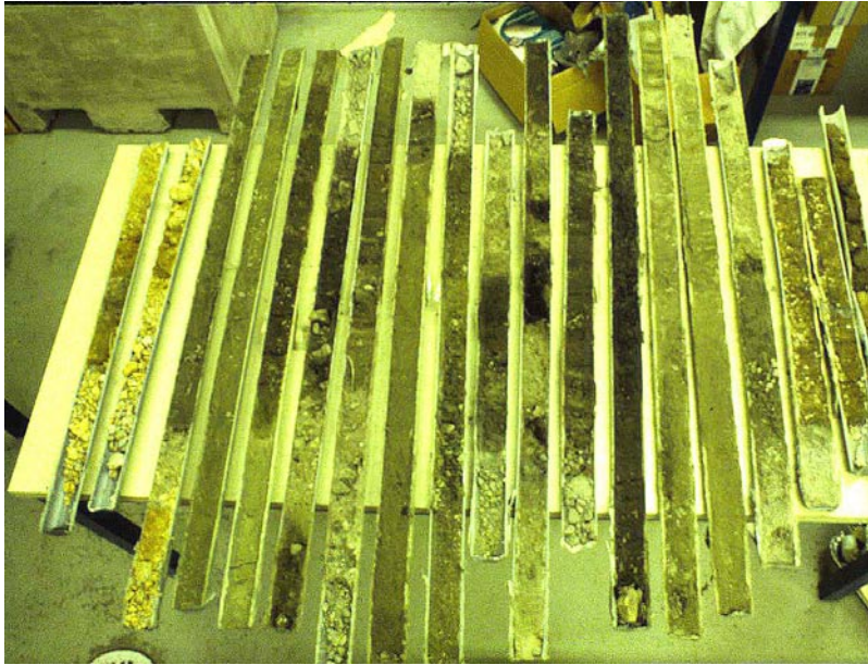
Figure 3-2. The Sokli B-series cores. The Eemian (MIS 5e) diatom gyttja deposit is on the right and the glacial till bed of MIS 3-2 age on the left.
