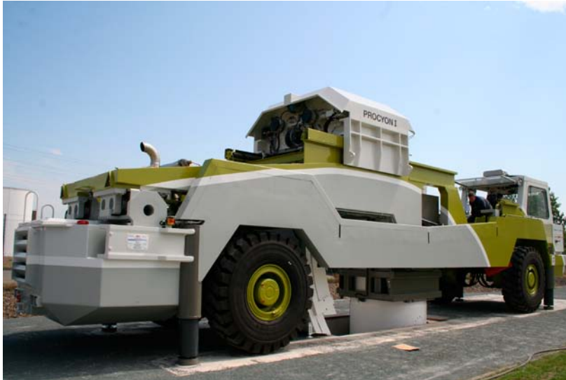
Figure 2-5. Newly developed deposition machine for handling of canisters in the final repository.
