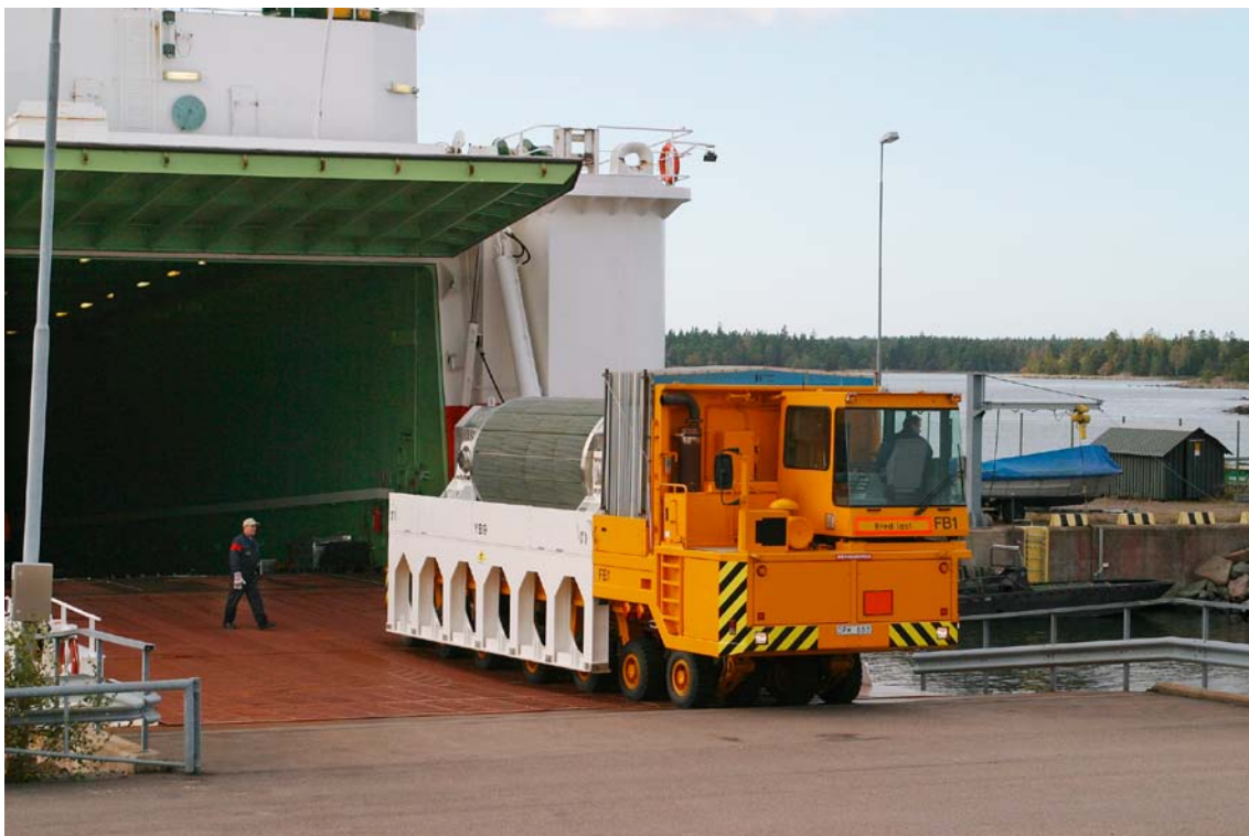
Figure 2-14. Terminal vehicle with transport cask.
