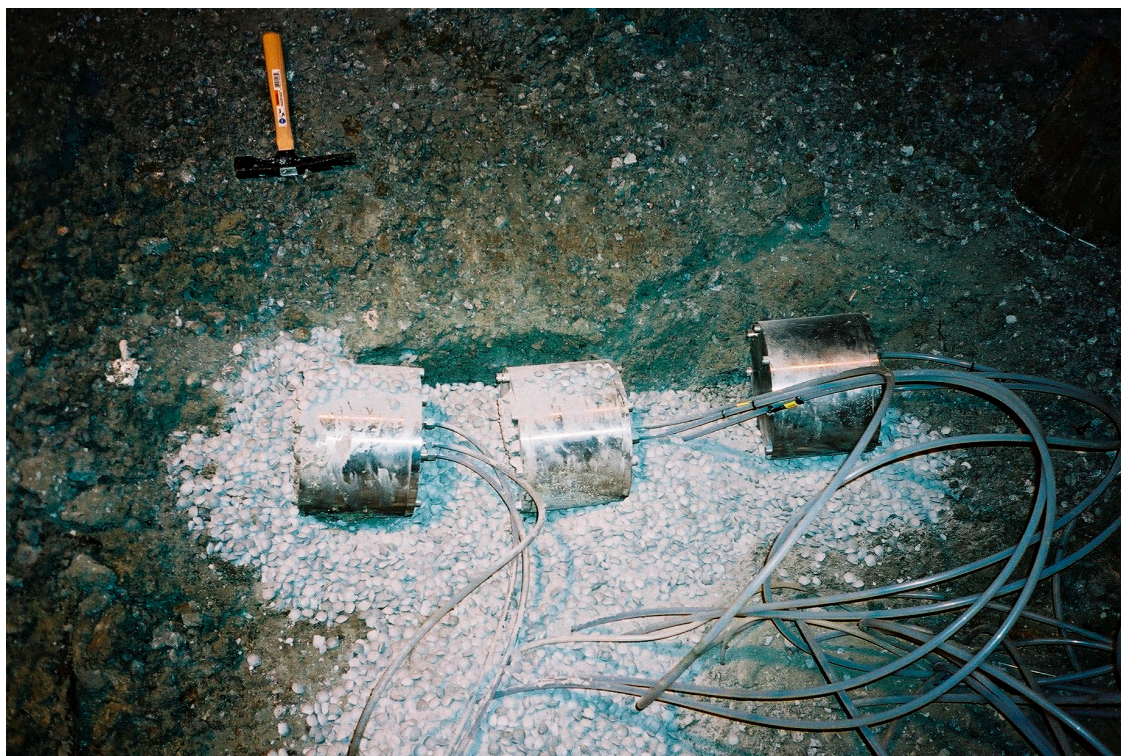
Figure 5-10. Vaisala amplifier boxes.
