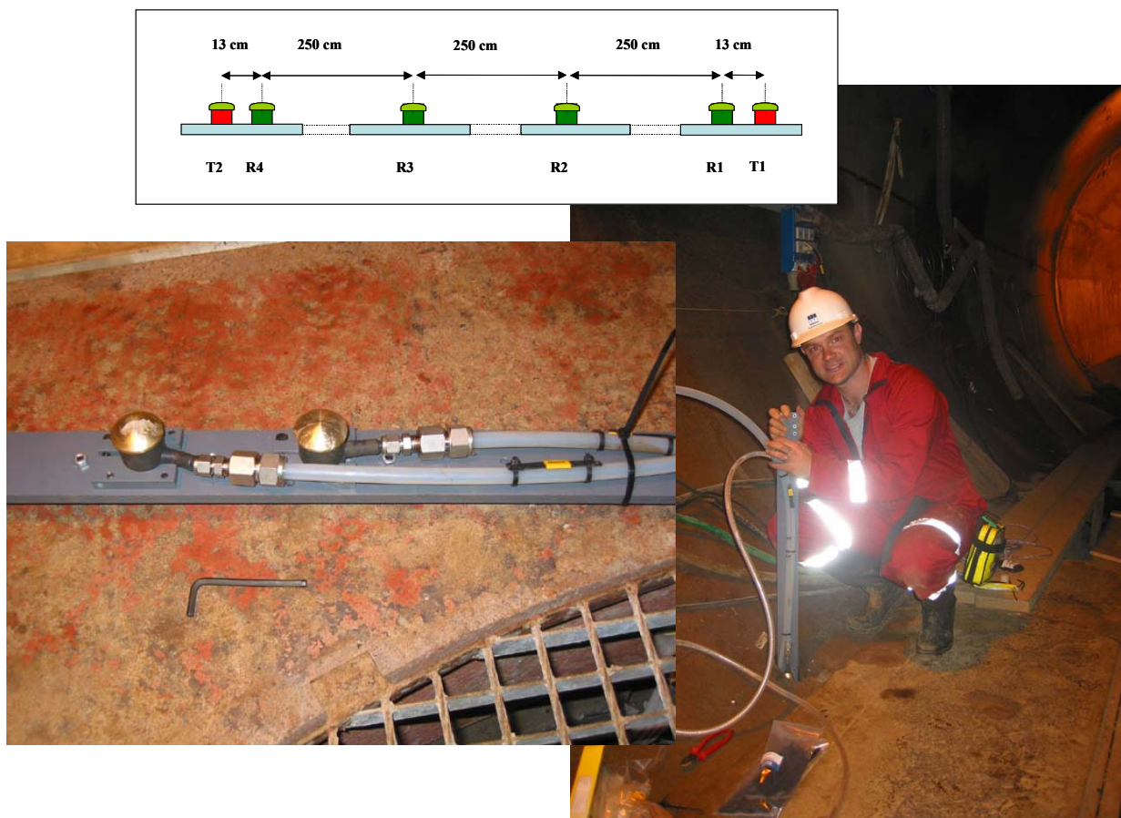
Figure 4-13: Top: Schematic diagram of the locations of all transducers on a single frame. Left: Photo of a section of the transducer assembly. Right: The transducer assembly during installation.
