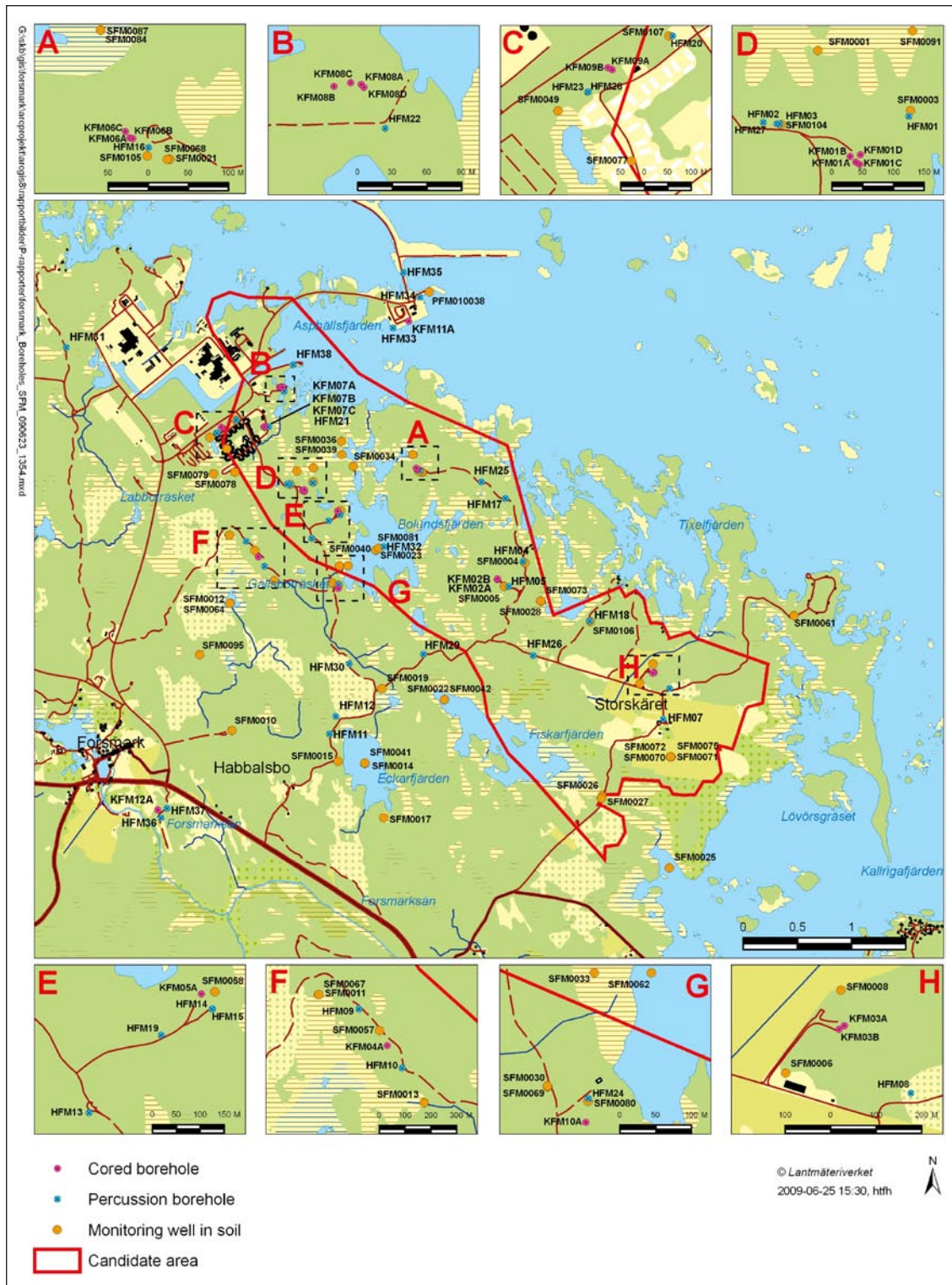
Figure 2-1. Overview of the Forsmark site investigation area with boreholes and surface-water level gauges.
