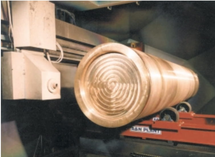
Figure 3-9. Electron beam welding of bottom on a copper tube.
