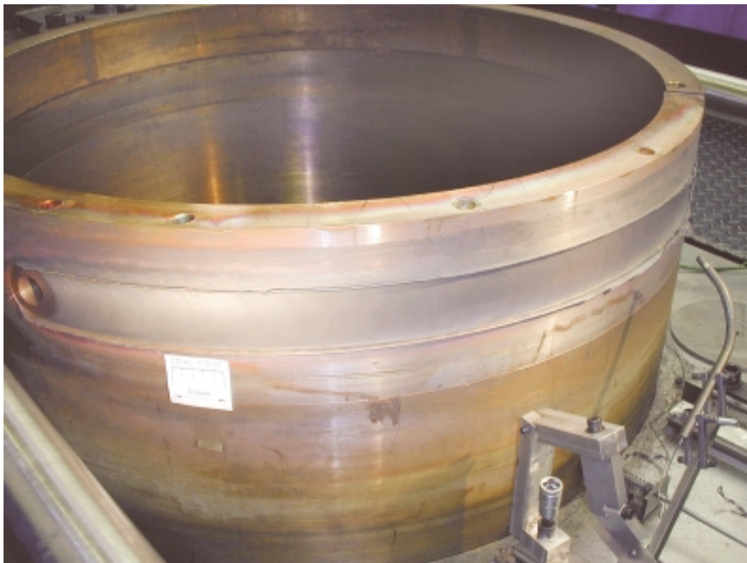
Figure 6-13. Weld around entire circumference.
