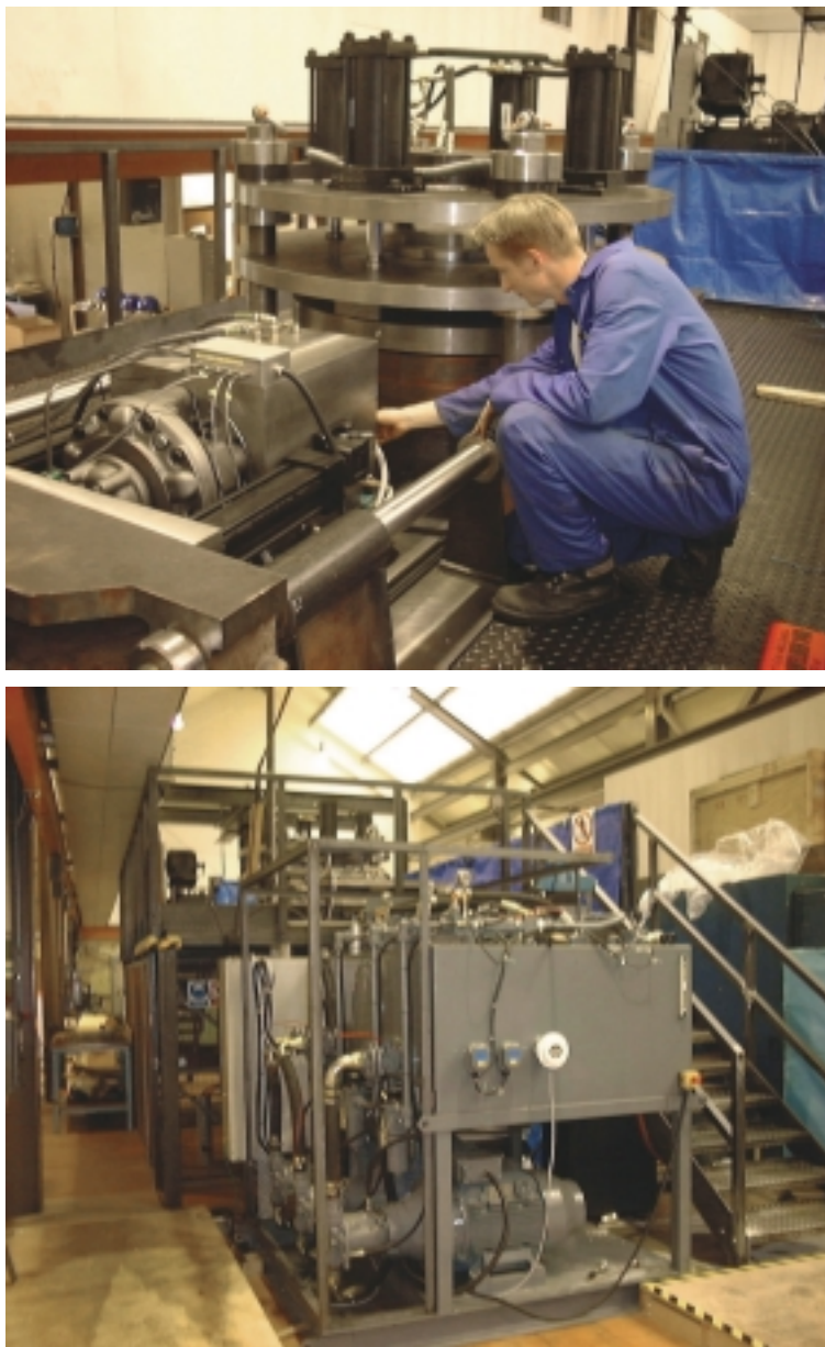
Figure 6-5. Machine for FSW of lids or bottoms on copper tubes.
