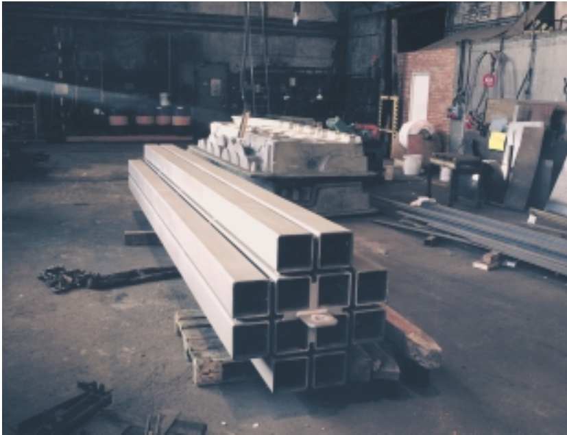
Figure 3-13. Welded cassette with 12 channels for BWR assemblies.
