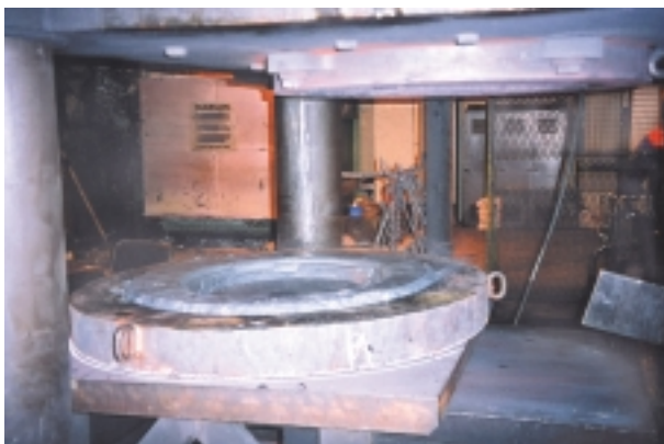
Figure 3-8A–C. Forging of blanks for copper lids and bottoms.
