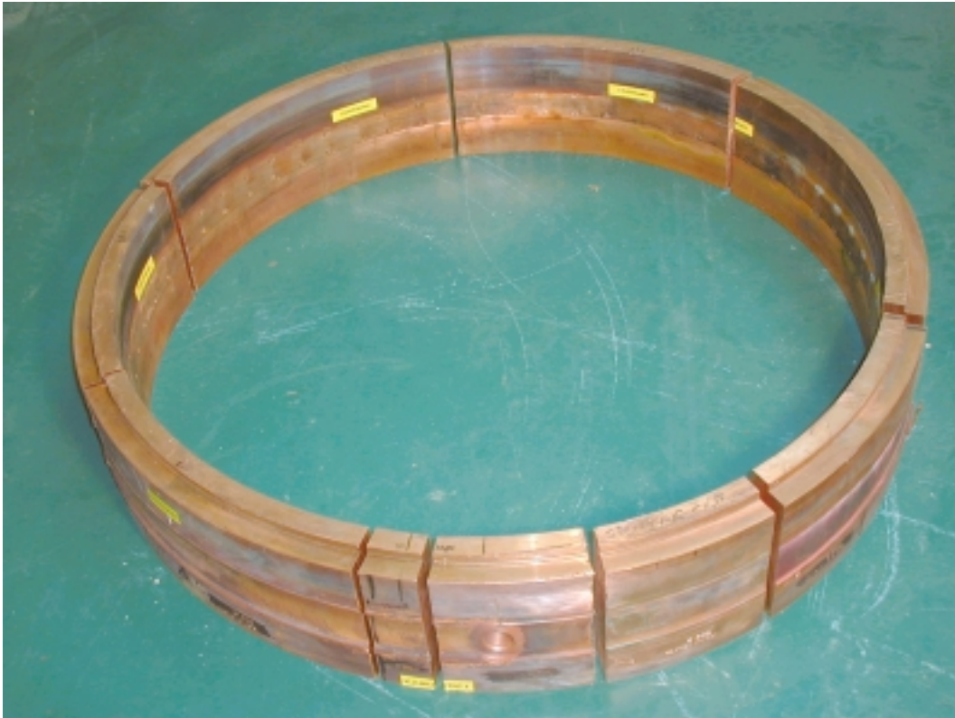
Figure 6-14. Weld CW 77 sent to IM for investigation.
