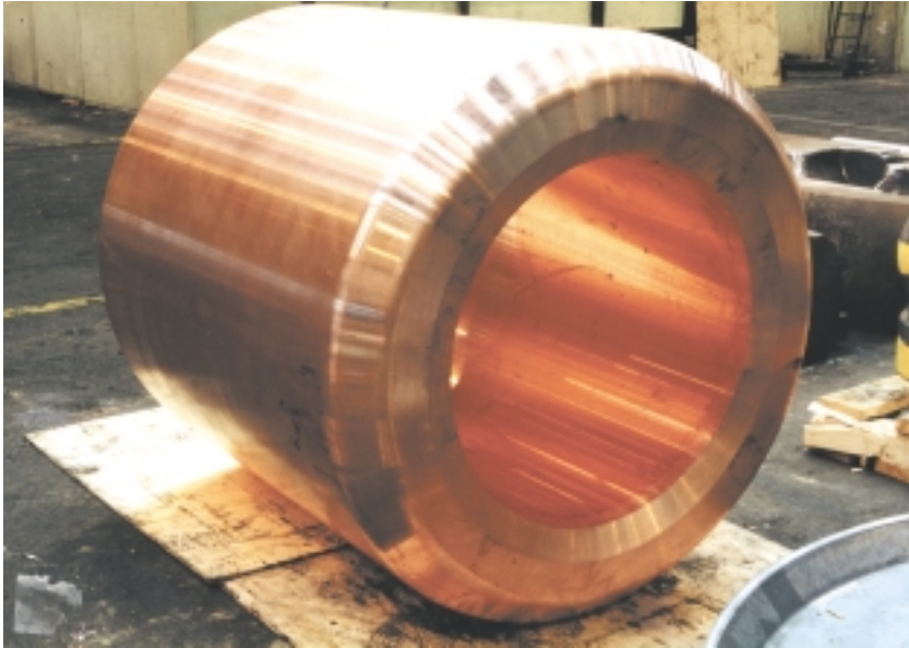
Figure 3-3. Hollow cylinder for extrusion.
