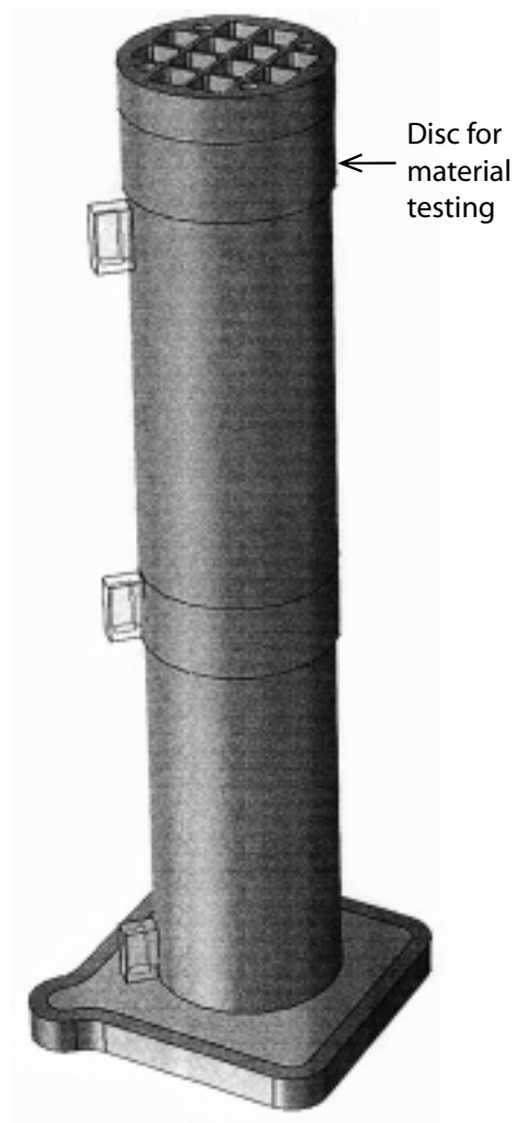
Figure 2-6. Cast-on test bodies near bottom, middle and top of insert. The extra length of the insert also enables a disc with a height of 200 mm to be cut out of the top part of the insert.
