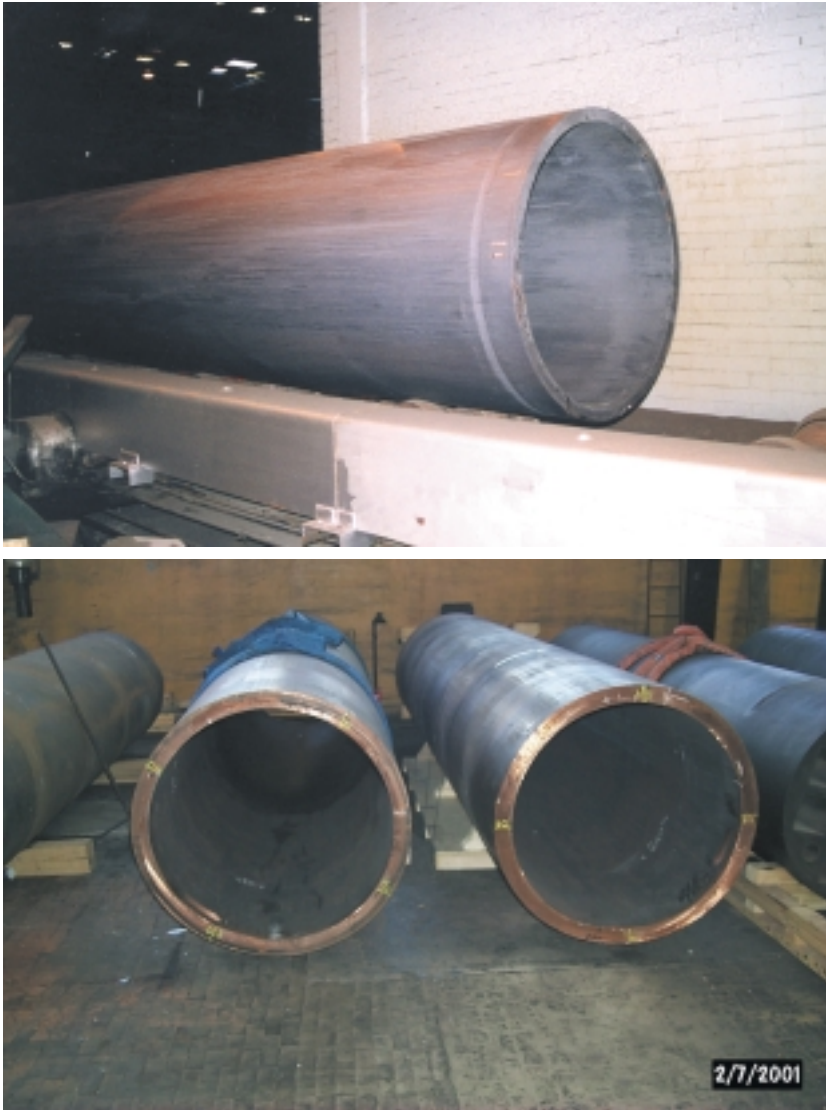
Figure 3-5. Extruded copper tube. At the top tube T 22 made for 30 mm wall thickness and at the bottom tubes T 23 and T 29, which will be machined to 50 mm wall thickness.
