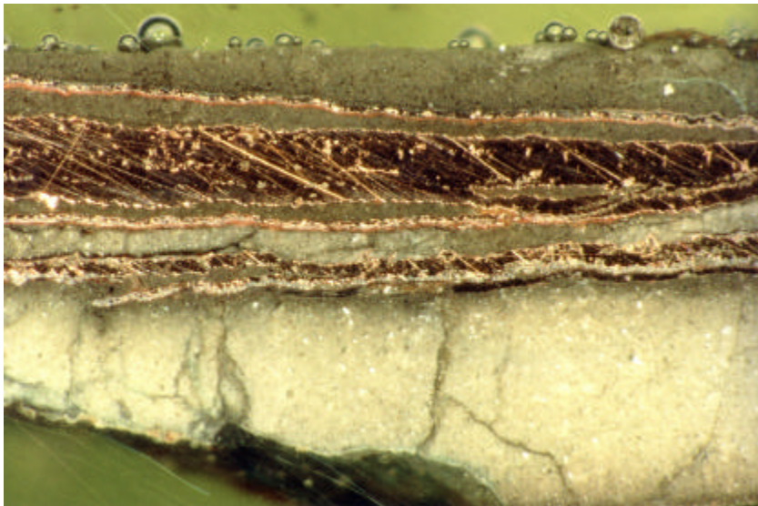
Plate 17. Detail of the right hand part of B3 showing the sub-parallel copper sheets. Field of view = 9 mm.
