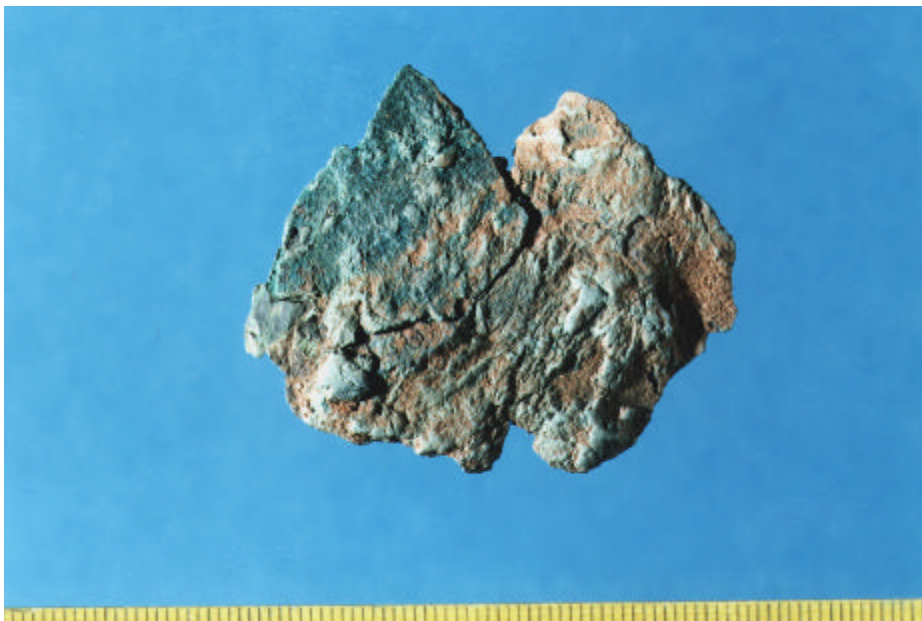
Plate 21. Copper plate B4, showing altered surface with fragments of grey siltstone still attached. Field of view = 25 mm.
