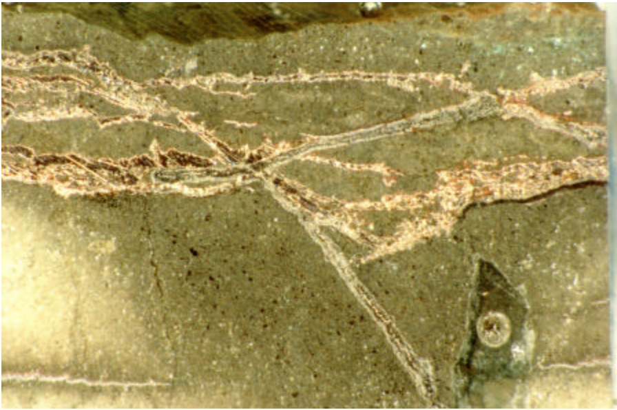
Plate 19. Detail of right hand side of B3 showing oblique nickel arsenide-enclosed copper sheets along 'shear planes' that disrupt the earlier 'horizontal' copper sheets. Field of view = 9.5 mm.
