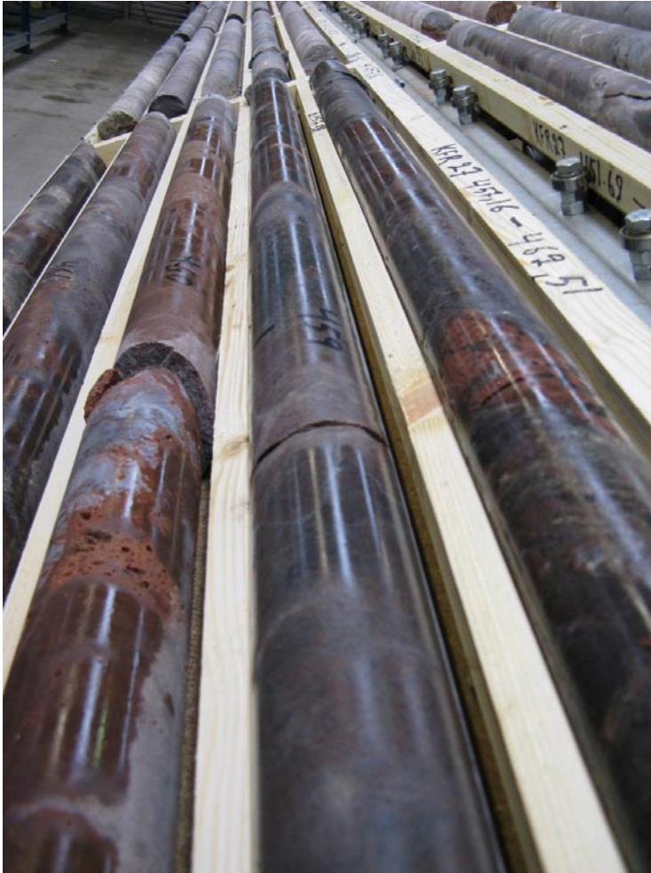
Figure 5-35. The core boxes were transported every morning during the drilling period to the core store-room, the so called Lentab facility. A simplified geological core mapping was performed, and afterwards all core boxes were photographed. A detailed core mapping (Boremap mapping) will be carried out after completion of drilling.
