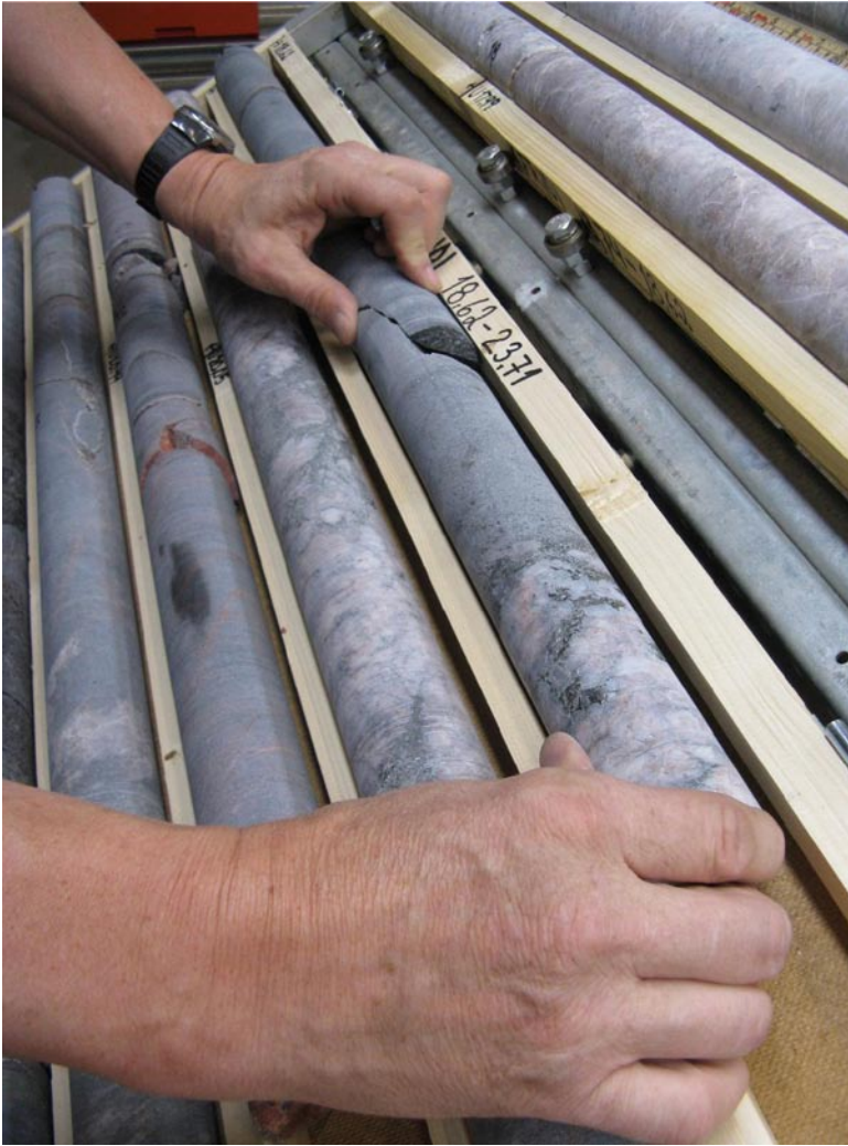
Figure 5-24. The core boxes were transported every morning during the drilling period to the core store-room, the so called Llentab facility. A simplified geological core mapping was performed, and afterwards all core boxes were photographed. A detailed core mapping (Boremap mapping) will be carried out after completion of drilling.
