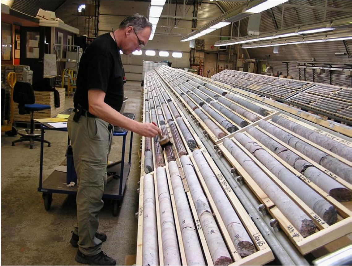
Figure 5-12. The core boxes were transported every morning during the drilling period to the core store-room, the so called Llentab facility. A simplified geological core mapping was performed, and afterwards all core boxes were photographed. Detailed core mapping, so called Boremap mapping, will be carried out after completion of drilling.
