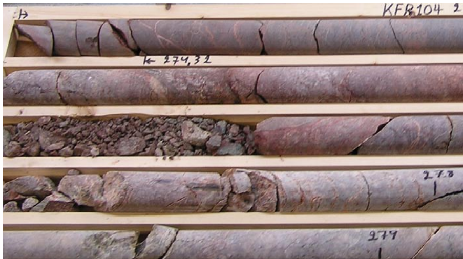
Figure 5-49. Image of the instable section in borehole KFR104.
