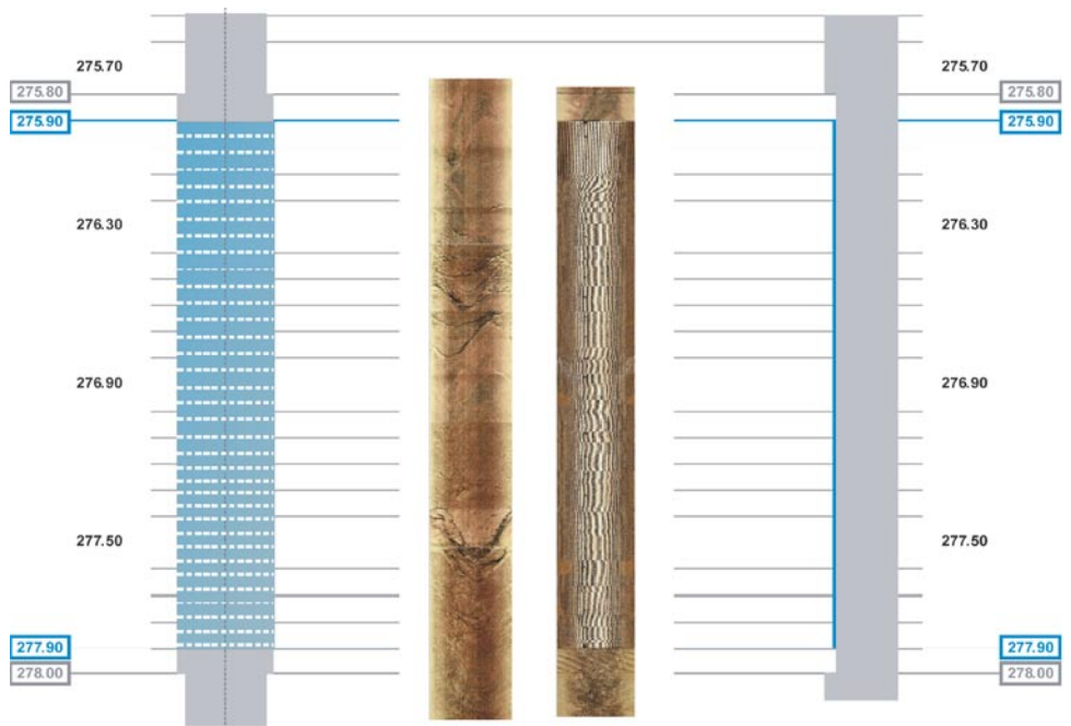
Figure 5-50. Schematic figure of the stabilized section in borehole KFR104 with BIPS –images of the borehole section, both before and after stabilization with the Plex system.
