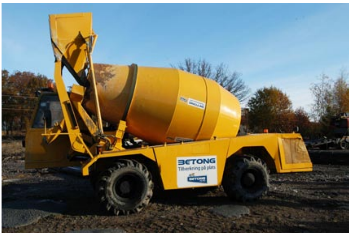
Figure 4-1. Truck mixer used in the factory test.
