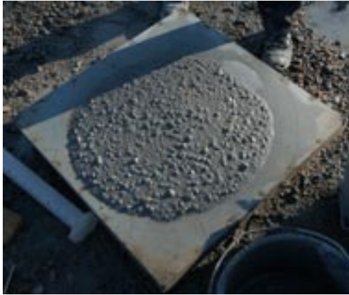
Figure 3-2. Slump flow test, note the evenly distributed coarse aggregate.
