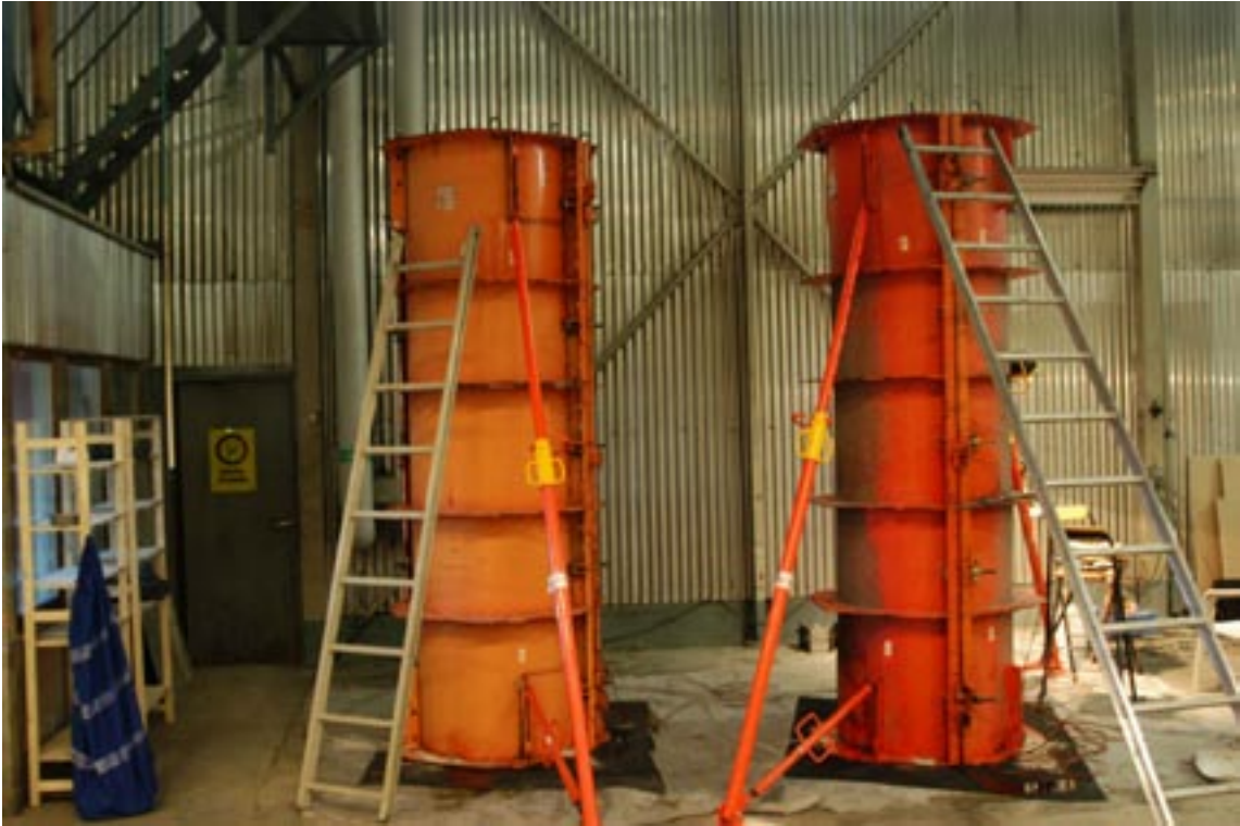
Figure 4-3. Two cylindrical steel moulds, diameter 0.85 m and height 3 m, instrumented with temperature gauges and one LVDT at the top to measure the settlement, were filled with low pH SCC.
