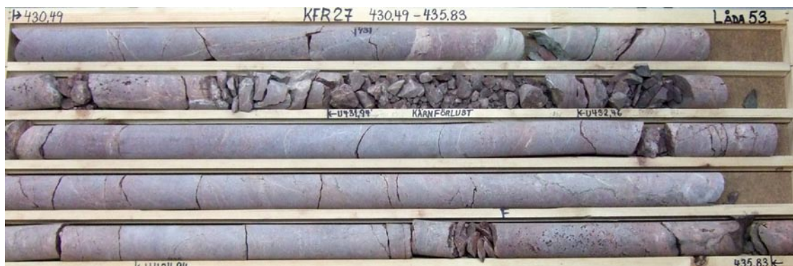
Figure 5-19. Image of the drill core at the instable section just below 430 m borehole length in borehole KFR27.
