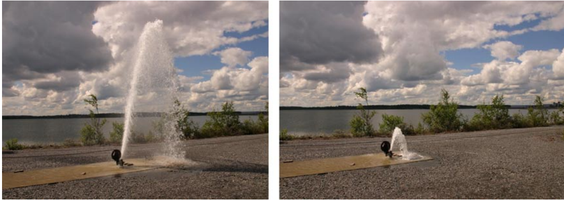
Figure 5-18. Illustration of nitrogen flushing. Nitrogen under a high pressure is forced through a hose to the bottom of the borehole. When the gas expands in the borehole, the mixture of flushing water and drilling debris is lifted up from the borehole bottom. When the supply of nitrogen is closed, the gas- and groundwater outflow ceases. The groundwater level has to recover before additional nitrogen flushing can begin.
