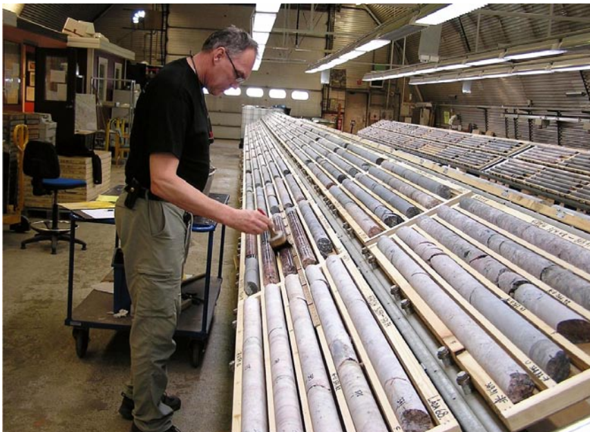
Figure 5-14. The core boxes were transported every morning during the drilling period to the core store-room, the so called Llentab facility. A simplified geological core mapping was performed, and afterwards all core boxes were photographed. A detailed core mapping together with analysis of BIPS-images, so called Boremap mapping, will be carried out after completion of drilling.
