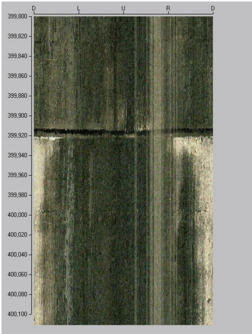
Figure 5-3. BIPS image from 399.80 to 400.10 m. A cut in the casing can be clearly seen at 399.92 m.
