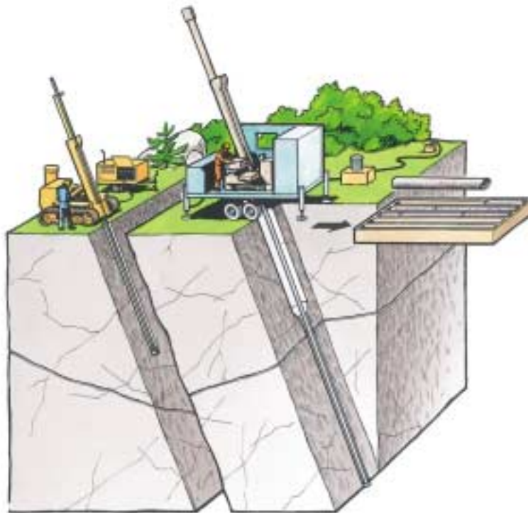
Figure 11-3. Shallower holes are normally percussion-drilled (at left in figure), whereby the rock is crushed to cuttings, while deep boreholes are core-drilled with a diamond drill bit, whereby the drill core is retrieved for geological mapping. The figure illustrates diamond drilling in accordance with the telescopic drilling method (see section on core drilling).
