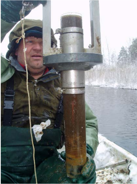
Figure 3-2. Compact, modified stainless steel “Kajak sampler” with 50–90 cm long metal-free polycarbonate tubes used for collecting sediment cores. Photo from Labboträsket, April 2008.
