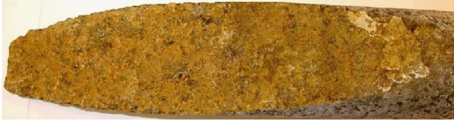
Photograph of sample KLX11D: 0.930–1.030 m (fracture surface with e.g. goethite).
