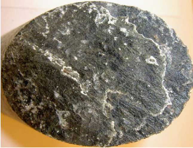
Photograph of sample KLX11D: 13.740–13.805 m (fracture surface with e.g. chlorite and calcite).
