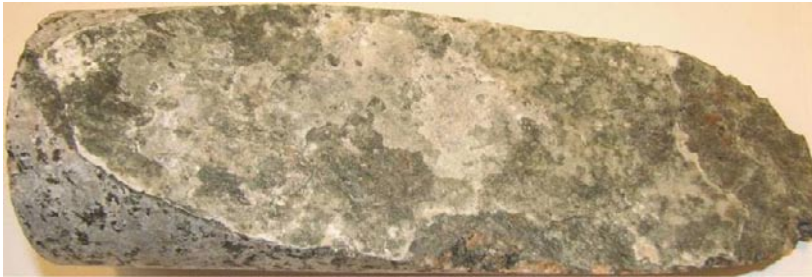
Photograph of sample KLX11E: 98.820–98.889 m (fracture surface with e.g. calcite and chlorite).
