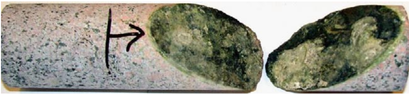
Photograph of sample KLX11E: 42.345–42.451 m (fracture surfaces with e.g. chlorite).
