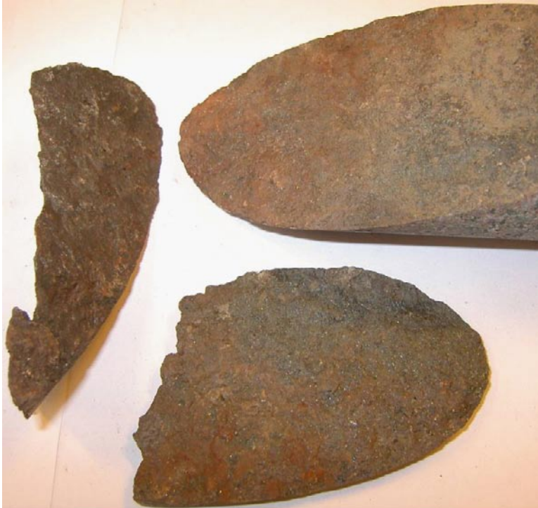
Photograph of sample KLX11E: 120.830–120.915 m (fracture surfaces with pyrite crystals on hematite-stained surface).
