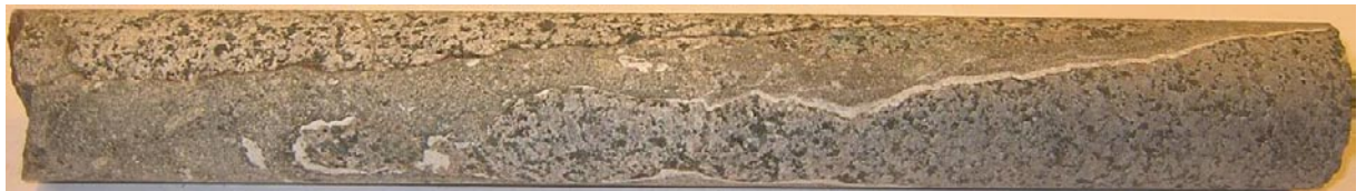
Photograph of sample KLX11D: 30.410–30.798 m (sandstone- and calcite-filled fracture).
