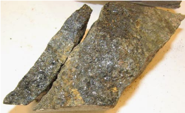
Photograph of sample KLX11E: 21.465–21.520 m (fracture surface with e.g. chlorite and goethite).
