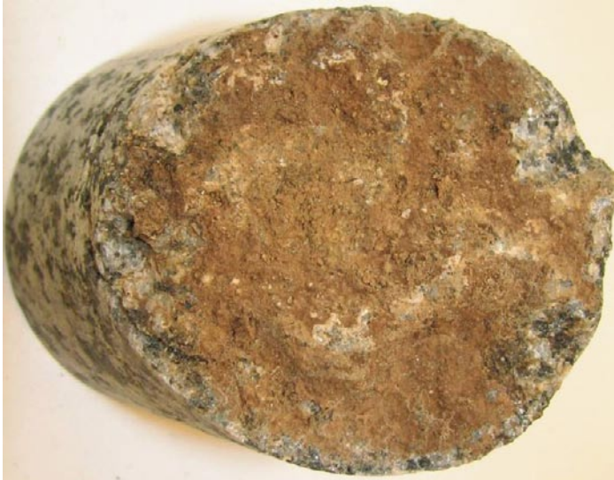
Photograph of sample KLX11E: 1.840–1.890 m (fracture surface with e.g. goethite).
