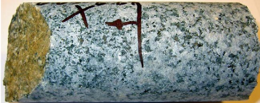
Photograph of sample KLX11F: 6.631–6.691 m (fracture surface with e.g. goethite).
