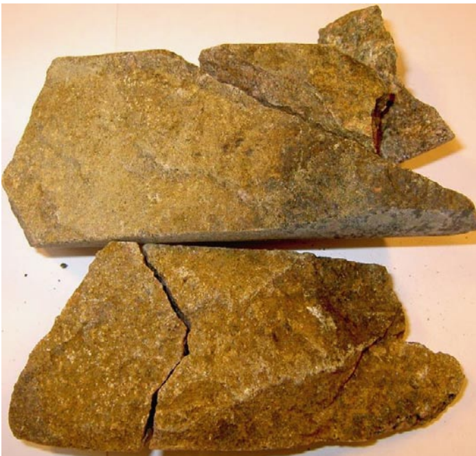
Photograph of sample KLX11F: 9.590–9.690 m (fracture surfaces with e.g. goethite).
