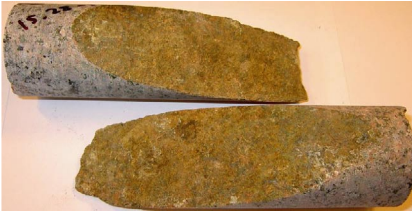
Photograph of sample KLX11F: 15.280–15.485 m (fracture surfaces with e.g. goethite and calcite).
