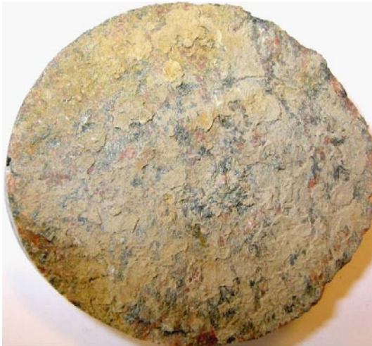
Photograph of sample KLX11D: 2.020–2.060 m (fracture surface with e.g. goethite).
