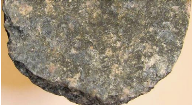
Photograph of sample KLX11C: 18.450–18.590 m (fracture surface with pyrite, chlorite etc).
