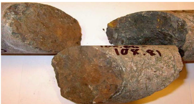
Photograph of sample KLX11D: 108.600–108.810 m (fracture surfaces with e.g. chlorite hematite and goethite).
