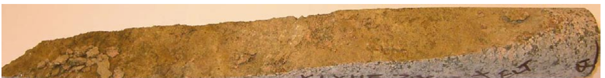
Photograph of sample KLX11F: 2.350–2.585 m (fracture surface with e.g. goethite).
