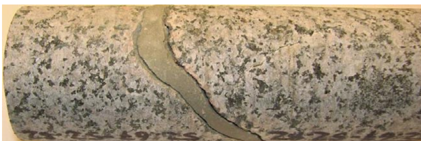
Photograph of sample KLX11C: 52.670–52.820 m (sandstone-filled fracture).
