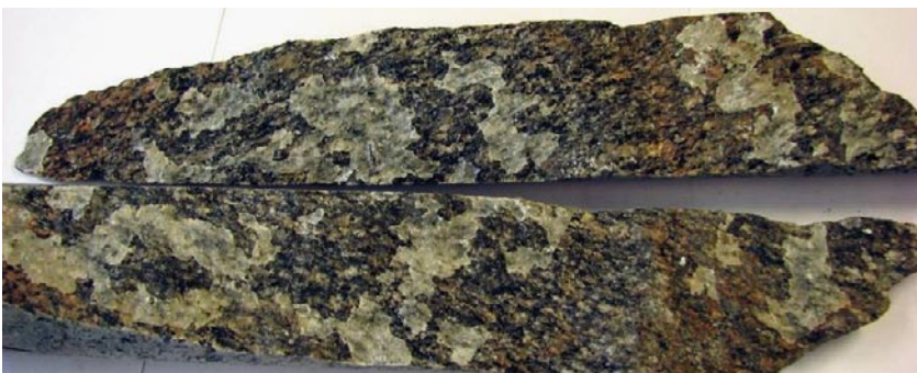
Photograph of sample KLX11E: 59.870–60.148 m (fracture surfaces with calcite).
