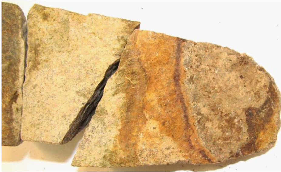
Figure 7-2. Typical appearance of goethite (brown colour) in a near surface open fracture. Sample KLX11B: 3.480–3.710 m.
