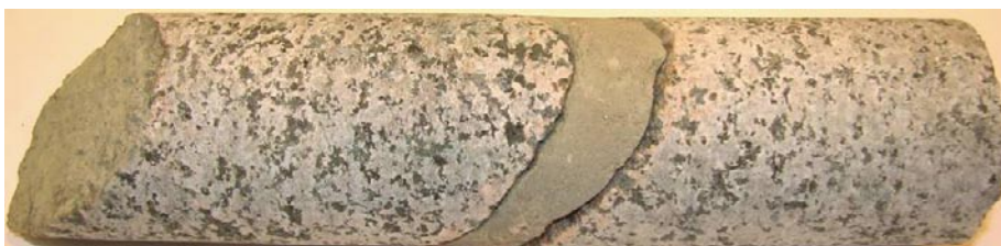
Photograph of sample KLX11C: 93.570–93.770 m (sandstone-filled fracture).
