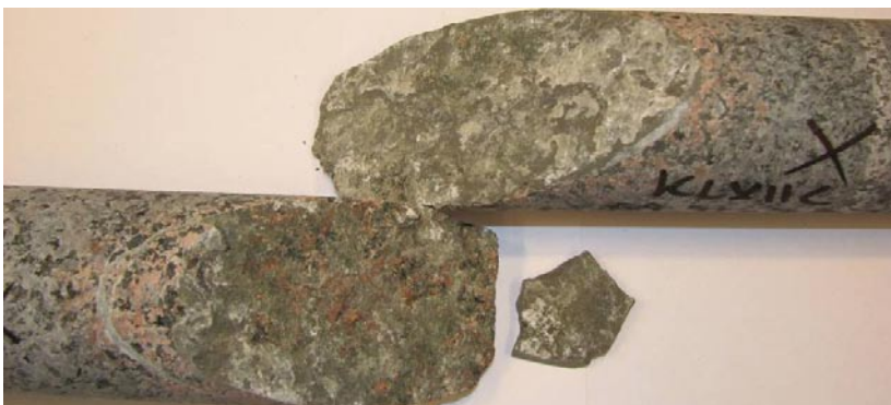
Photograph of sample KLX11C: 69.910–70.199 m (fracture coated by sandstone and nailhead shaped calcite).
