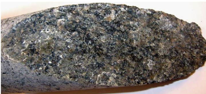
Photograph of sample KLX11F: 20.221–20.361 m (fracture surface with e.g. calcite).
