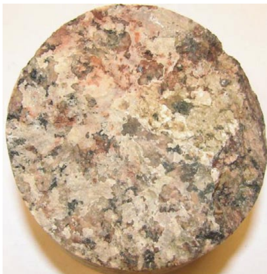
Photograph of sample KLX09F: 9.900–10.000 m (fracture surface).
