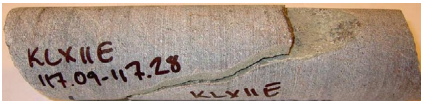
Photograph of sample KLX11E: 117.090–117.279 m (sandstone filled fracture).
