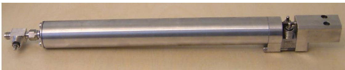
Figure A8-3. SKB stainless steel sampling cylinder (left: piston side, right: mounting adapter side).
