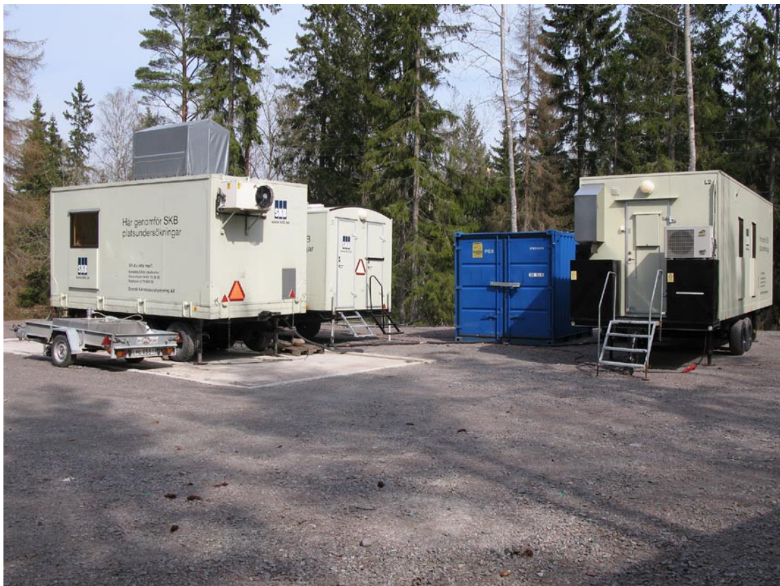
Figure 4-1. The mobile units used at KLX27A; (from left to right) hose unit with downhole equipment, laboratory unit, container for collecting the water from the borehole and a unit for computer work.
