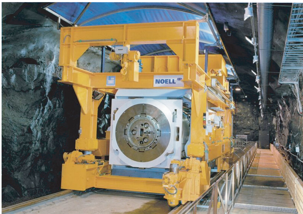
Figure 5: The current Prototype Deposition Machine dictate the current dimensions of the tunnels.
