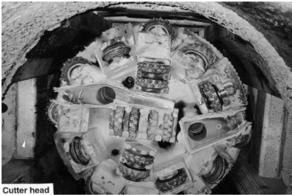
Figure 2-2. Boring machine Boretec DS 1.6 and its cutter head.
