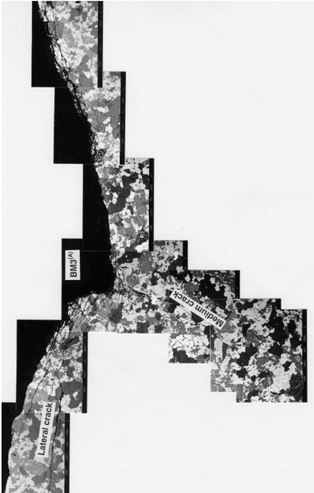
(c). The crater with a densely cracked zone, lateral cracks and medium cracks corresponding to BM3^{(A)} . The densely cracked zone is located around the crater (the black area in the left side) and it consists of many short cracks. The medium cracks are in the right side of the picture.
