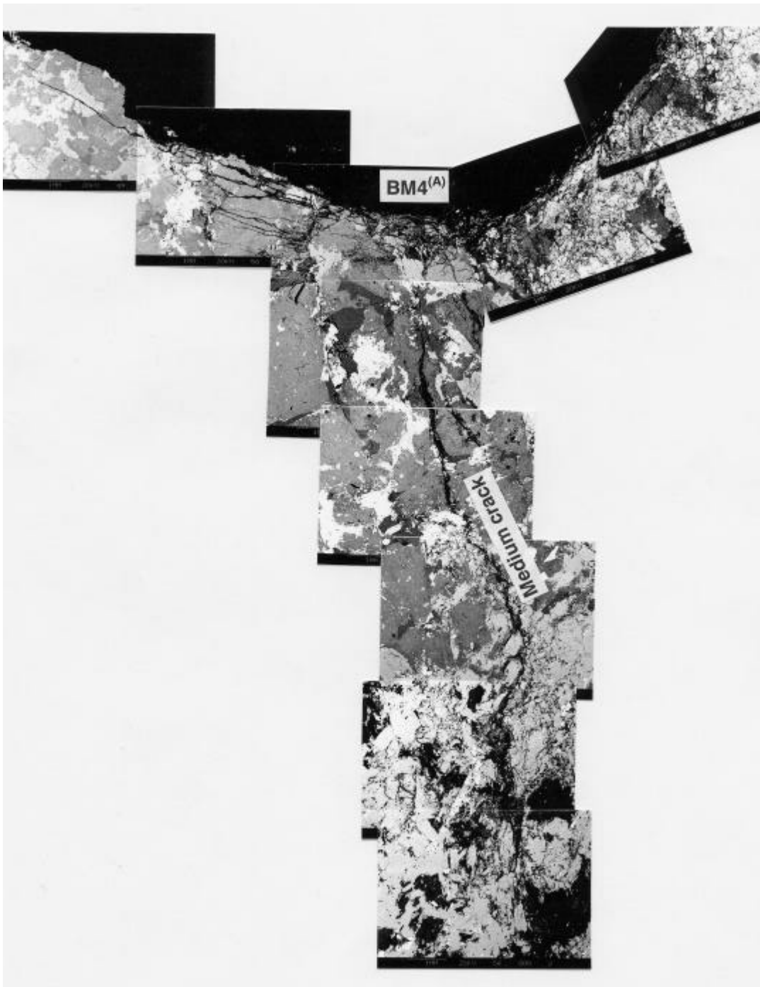
(d). The crater with a densely cracked zone and a long medium crack corresponding to BM4 (A) . The densely cracked zone is located around the crater (the black area in the upper part) and it consists of many short cracks. The medium crack is in the lower part of the picture.
