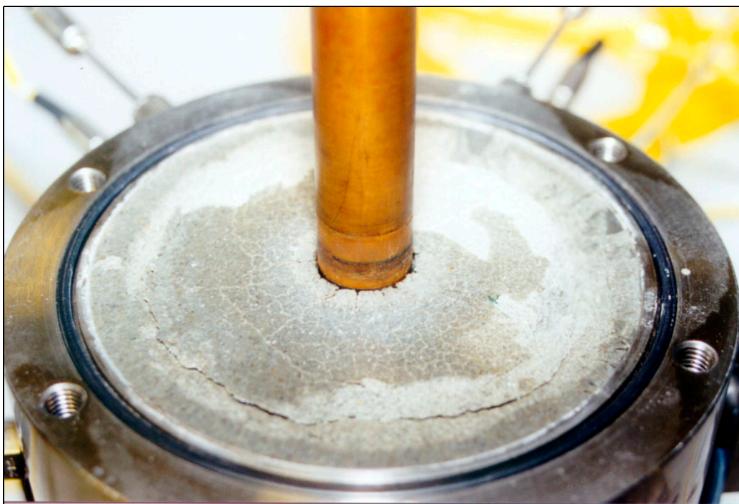
Figure 3-8 Photo from Test 2 showing the appearance at termination. Note the inner slot, which still exists
