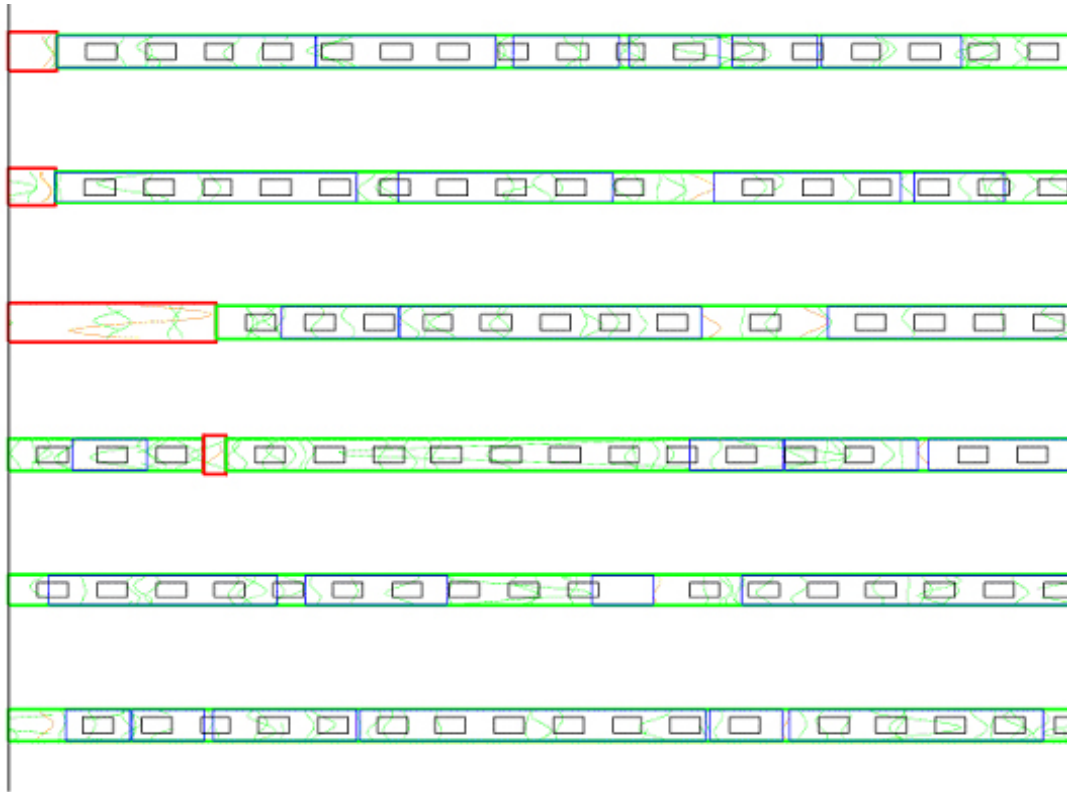
Figure 3-6. Detail of trace map. Red rectangles are compartment plugs. WCF traces with transmissivity greater than 2.65 \times 10^{-9} \text{ m}^2\text{s} (blank threshold) are shown in red, all other traces are in green. Blue rectangles show dry zones.
