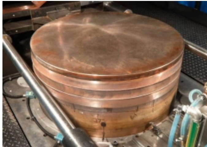
Figure 7. A complete circumferential friction stir welded canister.
