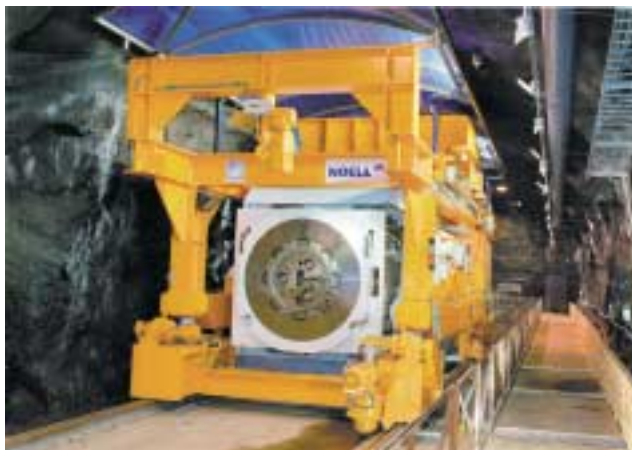
Figure 4-8. Picture of the deposition machine in the demonstration tunnel at Äspö.
