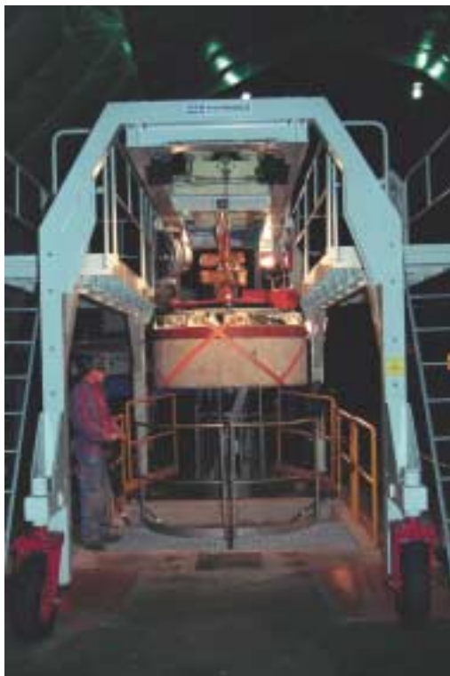
Figure 4-9. Photo of the gantry crane for handling of the compacted buffer material with handling tool for buffer material during testing in June 2000.
