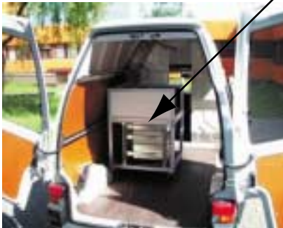
Figure 3-37. Equipment for Laser-induced Breakdown-Detection (LIBD) of colloids (upper picture). The equipment is installed in a van in order to allow mobility and on-line measurements (lower picture).
