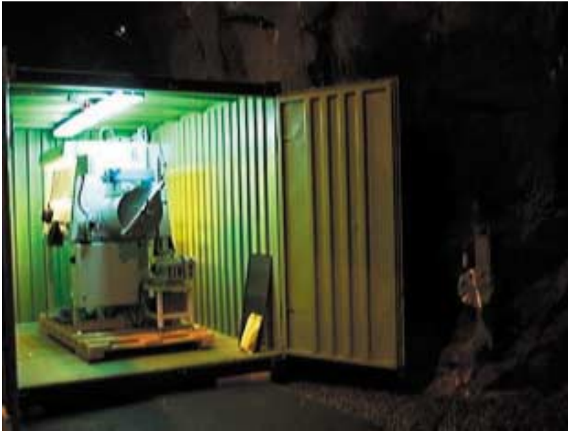
Figure 6-26. INE glovebox installed in a container close to CHEMLAB II drillhole (right).
