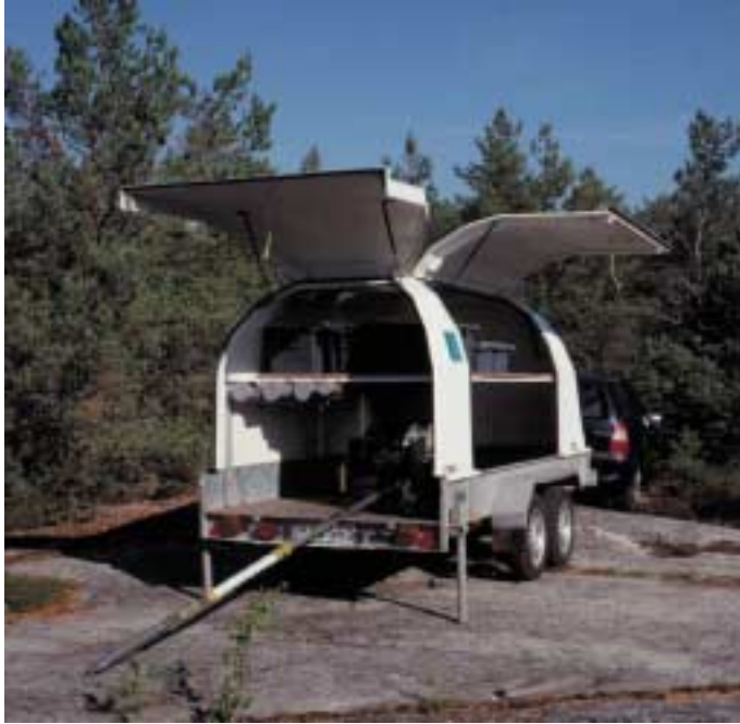
Figure 6-3. Posiva Flow Log was used in flow measurements in borehole KLX02 at Laxemar.
