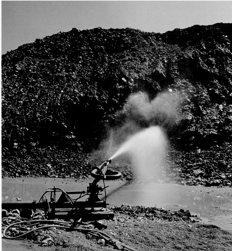
Figure 4-4. A commonly used application of the high pressure hydrodynamic technique, pressure less than 100 bar.
