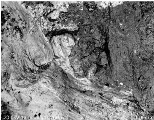
Back-scattered SEM-image of two kinds of mixed layer-clay; one Fe-rich (bright) and one Mg-rich (dark). Sample KLX08: 465.10–465.14 m.
