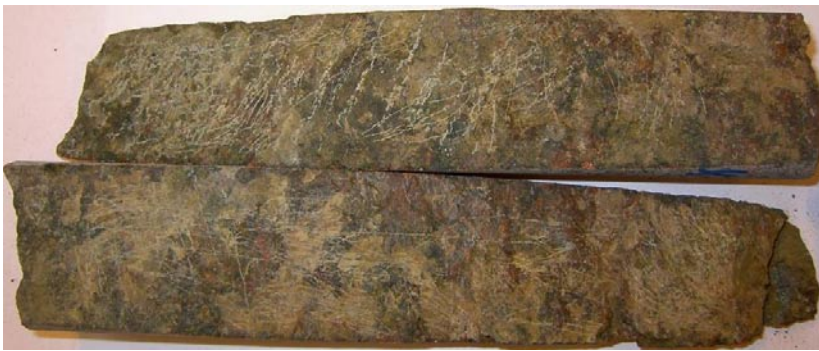
Photograph of the fracture surfaces of drill core sample KLX07B: 4.85–4.85 m.
