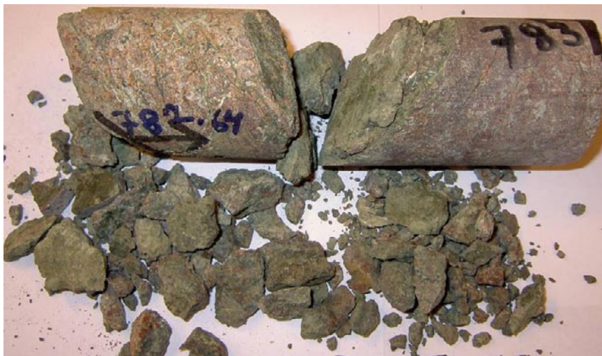
Photograph of drill core sample KLX07A: 782.64–782.83 m.
