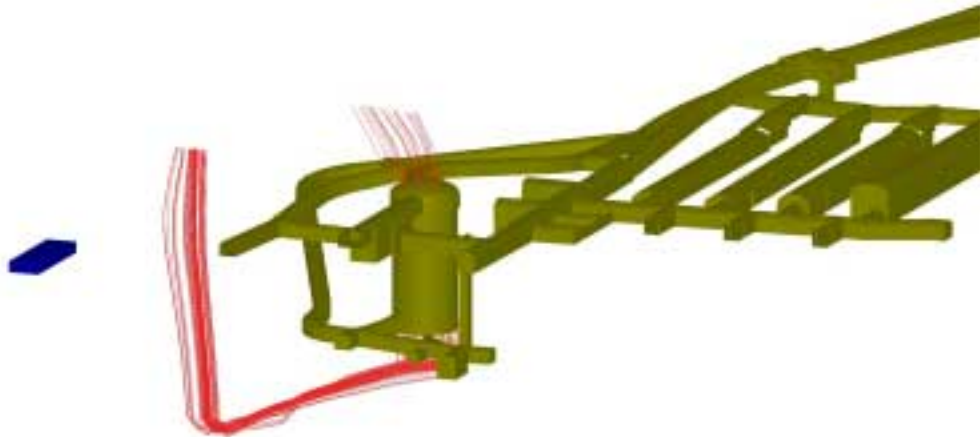
Figure 12.3 Well-case H. The major flow routes from the SILO, at time equal to 5000 AD. The well is at the centre of the blue box.
