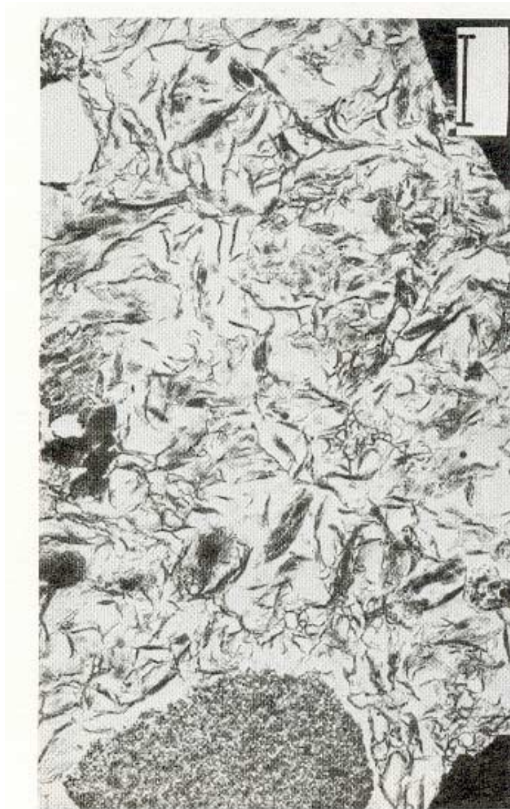
Figure 3-6. Transmission electron micrograph of stacks of montmorillonite lamellae forming a very open structure of cardhouse type (Bar is 1 \mu\text{m} ). Sample from the Pacific floor with 81 % clay content, mostly smectite, and a void ratio of 3.5 (bulk density about 1300 \text{ kg/m}^3 ). A zeolite aggregate is seen at the base. Micrograph by R H Bennett.
