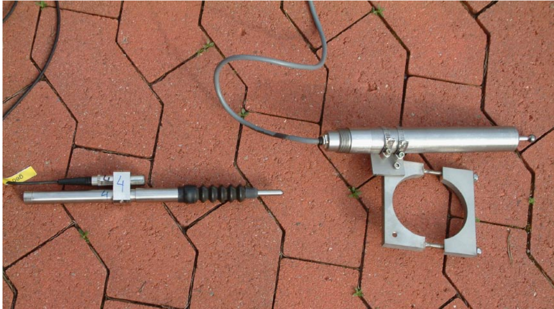
Figure 4-1. Photograph of the two LVDT types. Left the long range model and right the short range model. The short range model is attached to the equipment that will be mounted on the supporting construction consisting of vertical steel pipes along the pillar wall.
