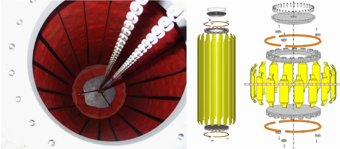
Figure 3-6. Left figure: the confinement equipment that will host the rubber bladder membrane, right: Microstation drawing of the equipment. The load bearing textile straps are orange/red in the construction and yellow in the drawing.
