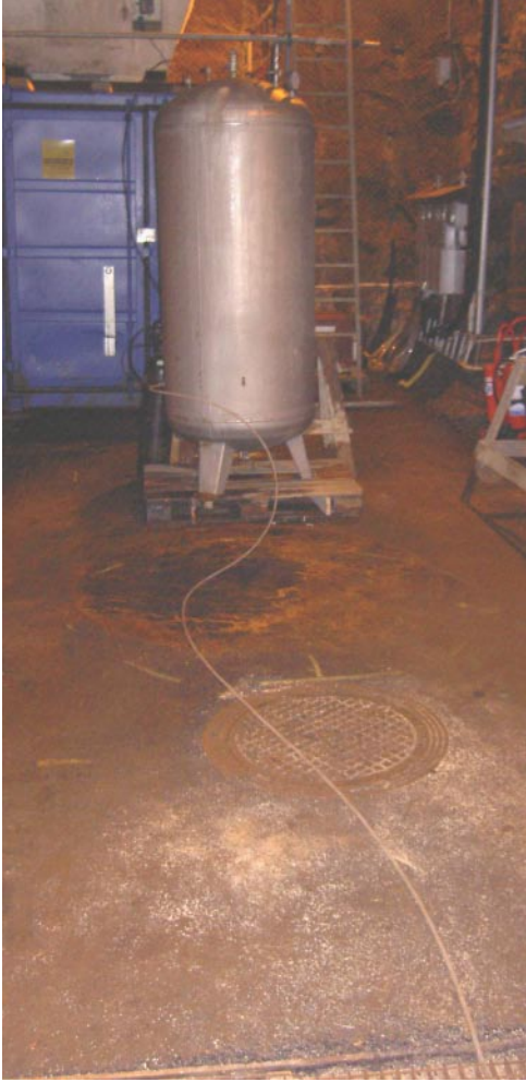
Figure 3-9. Photograph of the pressure vessel and the accompanying gas tube. The flexible Tecalan tube in the photograph is connected to the bladder via the top steel lid and ensures the pressure in the bladder even if there is a small water leakage through the sealing around the man-hatch in the lid.
