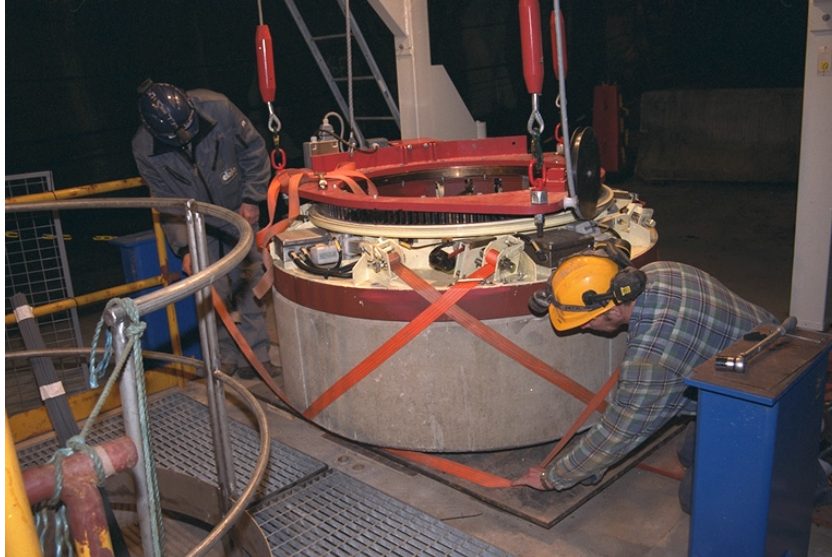
Figure 4-1 A block (in this case of concrete) is being attached to the gripping device
