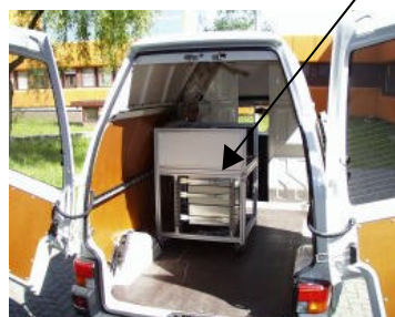
Figure 3: Equipment for Laser-induced Breakdown-Detection (LIBD) of colloids (upper picture). The equipment is installed in a van in order to allow mobility and on-line measurements (lower picture).
