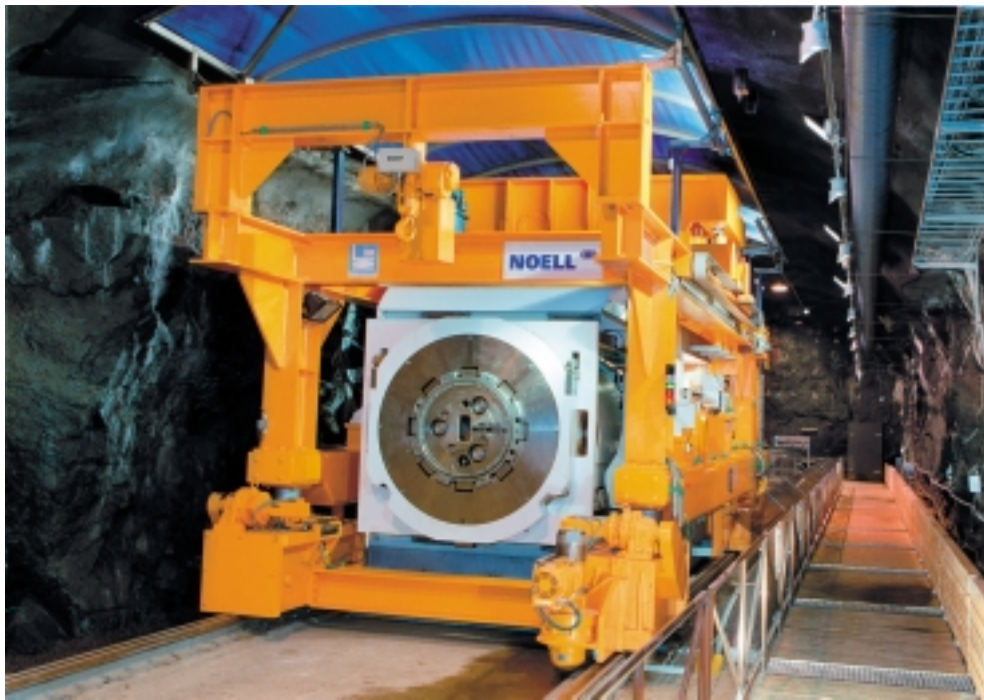
Figure 6-7. The current version of the deposition machine in the demonstration facility in the Äspö HRL. The radiation protection tube in which the canister is transported up to the deposition hole can be seen in the middle.
