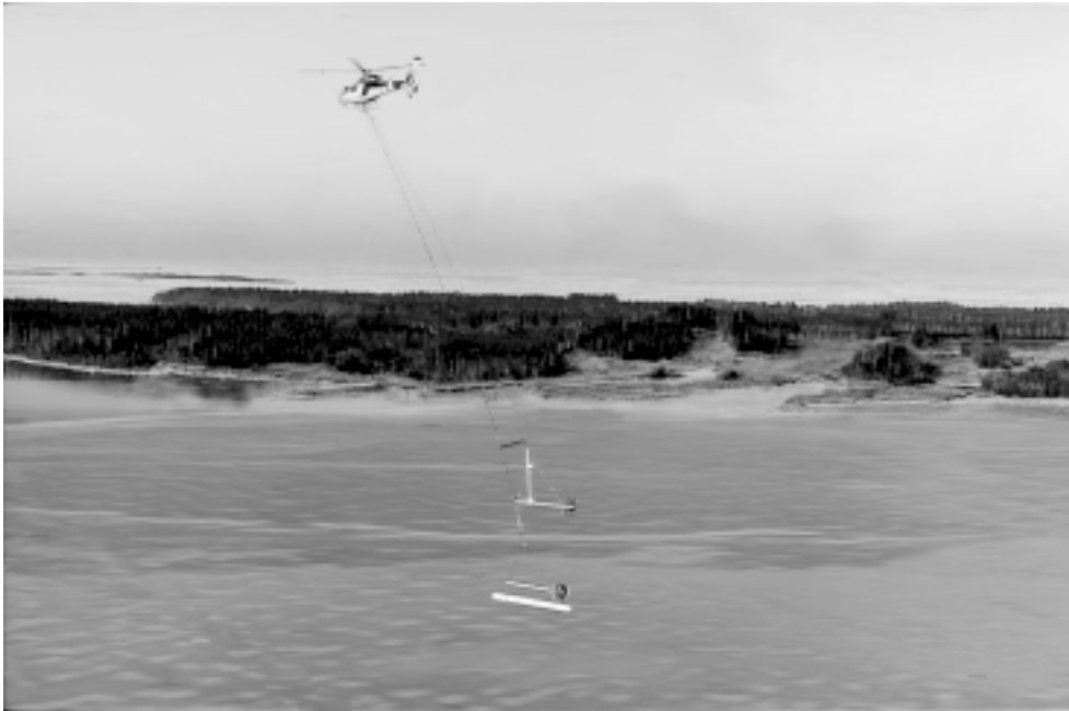
Figure 13-6. Geophysical measurements from a helicopter. Instruments that record the magnetic and electrical properties of the bedrock are placed in measuring probes suspended underneath the helicopter. (Photo from measurements in Finland, photo-montage.)
