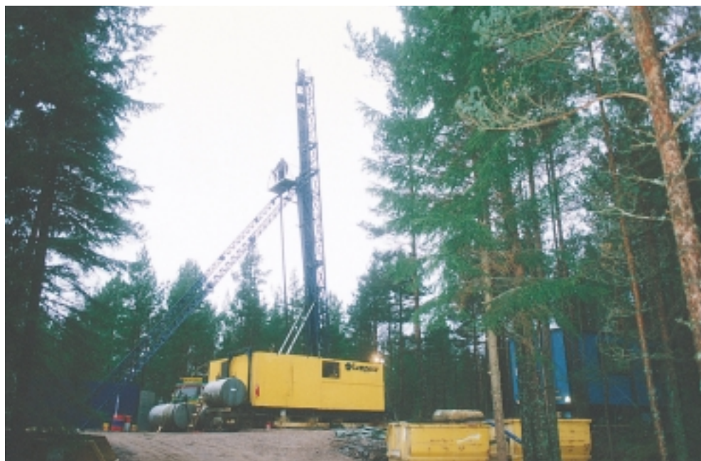
Figure 13-7. Example of worksite for core drilling.
