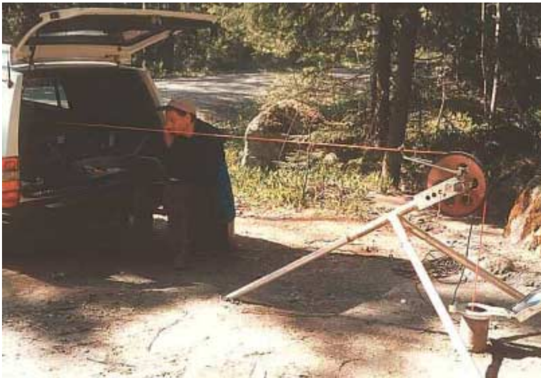
Figure 3-3. Measurement of borehole 1. The measuring wheel and the fibre optic cable can be seen in the picture.
