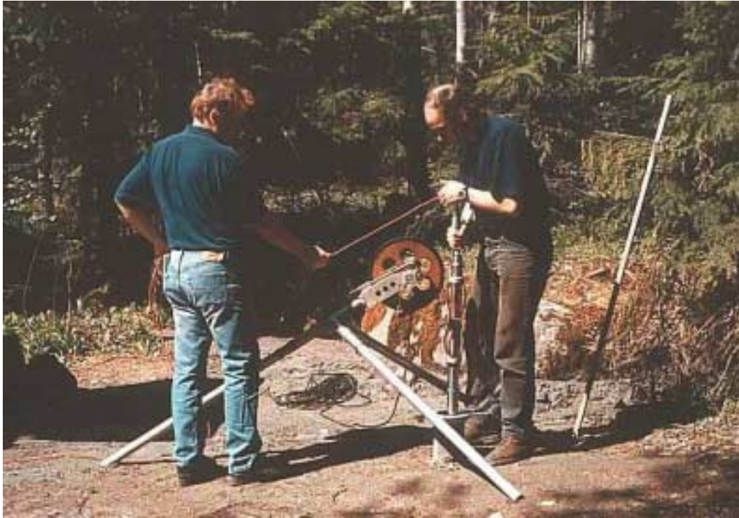
Figure 2-2. The vertical borehole 1 at the Boda site. The BIPS probe is lowered into the borehole. Please note the centralizers on the probe.
