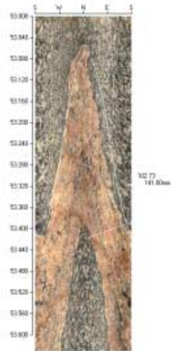
Figure 3-24. The pegmatitic veins are clearly oriented E/70–80°.
