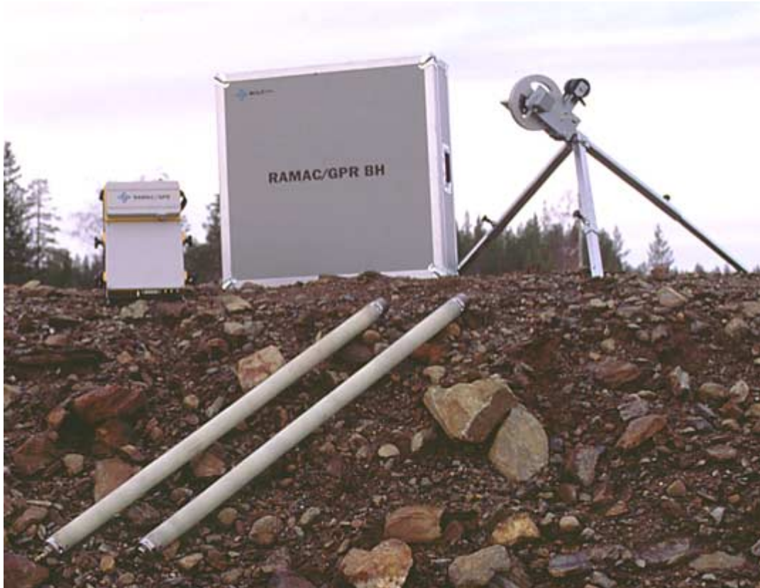
Figure 3-1. Picture of main parts of the RAMAC/GPR borehole radar system. Transmitter and receiver antennas in the front, control unit to the left, and measuring wheel to the right. Large box in the middle is the transport box.
