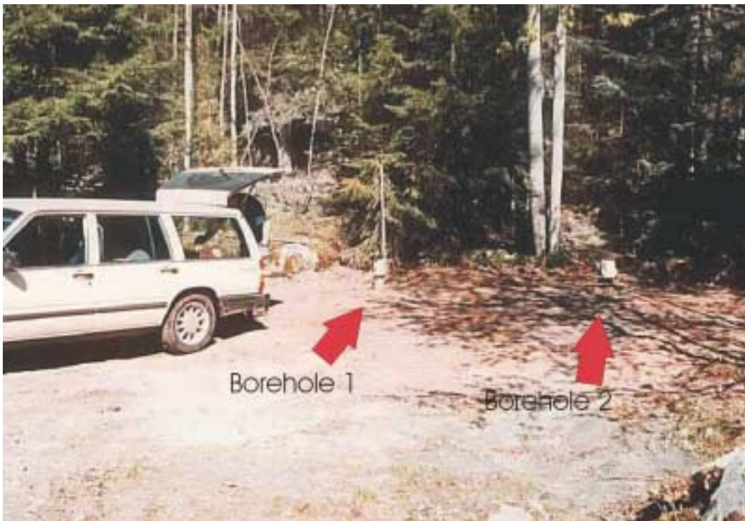
Figure 2-3. The vertical borehole 1 (to the left) and the dipping borehole 2 (to the right) at the old parking lot. Borehole 2 is directed into and under the cave area.
