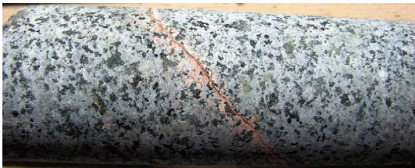
Figure 7-4. Fracture sealed with laumontite of Generation 3. Parts of the wall rock have red-stained plagioclase and/or plagioclase replaced by laumontite. Photograph is from a section at about 139.65 m (not sampled here).
