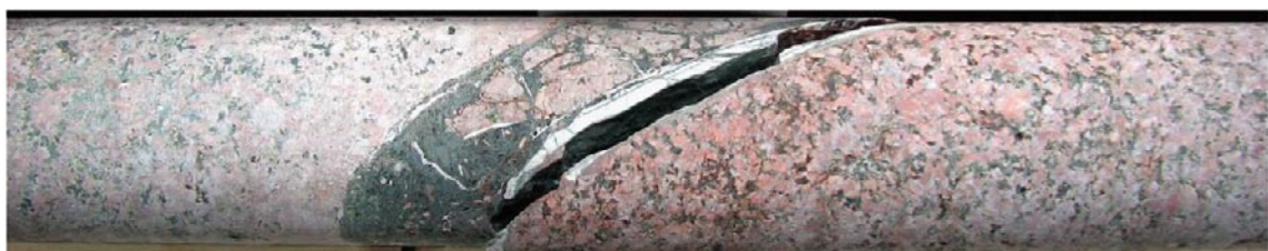
Figure 4-2. Red-stained wall rock adjacent to a reactivated fracture (filled with e.g. chlorite [green] and calcite [white]).
