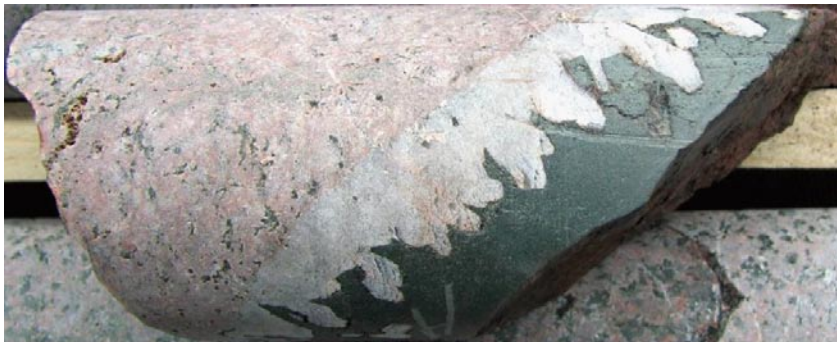
Figure 7-3. Chlorite (green) and quartz (greyish white) of Generation 3. The wall rock is red-stained due to hydrothermal alteration. Photograph is from a section at about 379–380 m (not sampled here).
