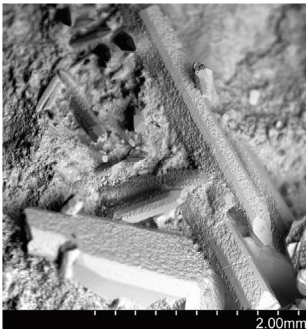
Figure 7-9. Back-scattered SEM-image of needle shaped calcite in sample KLX15A: 262.956–263.046 m.
