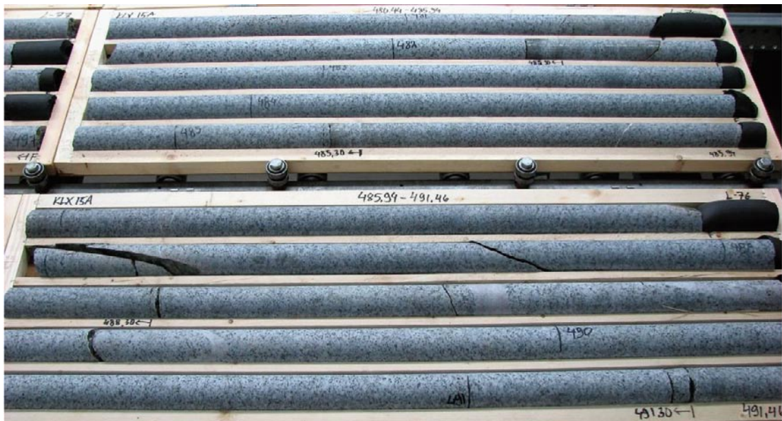
Figure 4-1. The drill core is dominated by sections with low amounts of fractures and relatively fresh quartz monzodiorite wall rock, here exemplified by section KLX15A: 480.44–491.46 m.
