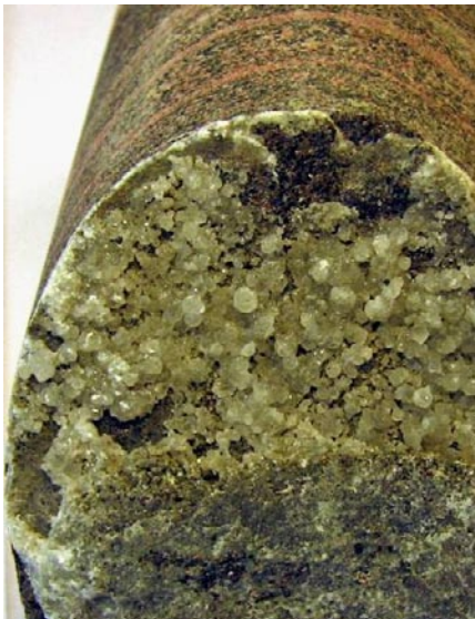
Photograph of the one of the fracture surfaces of sample KLX17A: 315.479–315.759 m. The surface is mainly coated by equant calcite crystals.
