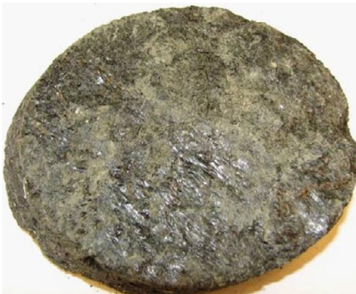
Photograph of one of the fracture surfaces of sample KLX17A: 426.100–426.360 m, showing a smooth, slickensided chlorite/clay mineral-dominated fracture coating.
