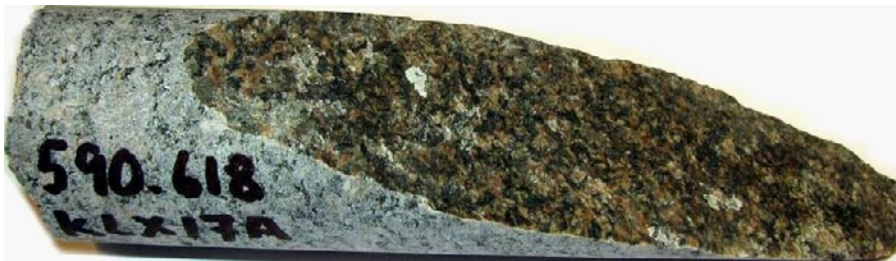
Photograph of the fracture surface of sample KLX17A: 590.652 –590.766 m. Gypsum is present along with apophyllite as a thin bright grey coating.
