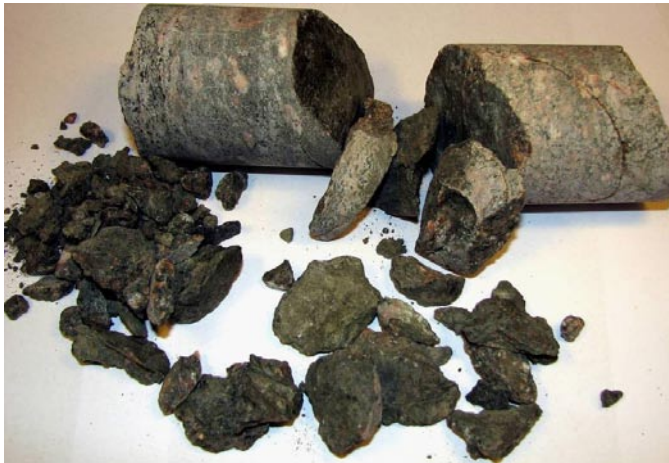
Photograph of the highly fractured drill core sample KLX17A: 423.250–423.450 m.
