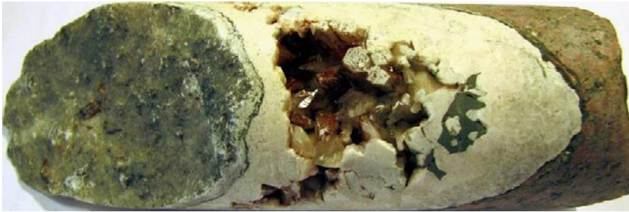
Photograph of sample KLX19A: 412.430–412.531, showing a fracture partly sealed by calcite (white, mostly scalenohedral, sometimes coated by hematite) and chlorite (green).
