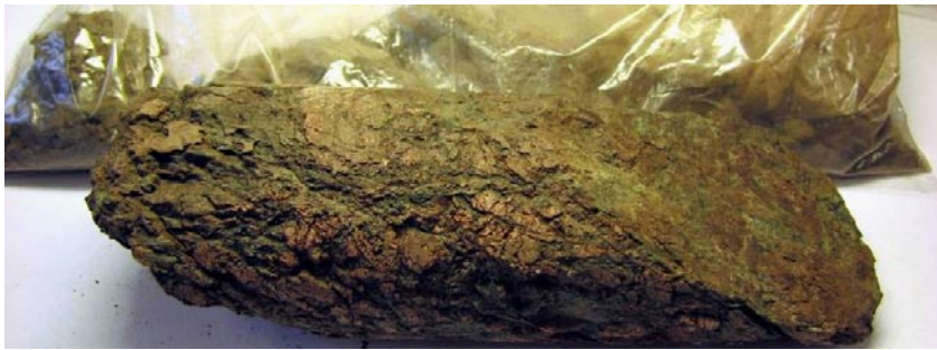
Photograph of sample KLX13A: 494.770–494.871 m. High amount of fine-grained material is contained in the plastic bag. The rock is highly fractured and consists of cataclasites of different grades.
