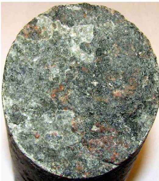
Photograph of the fracture surface of sample KLX17A: 449.800–449.880 m. Gypsum is present along with apophyllite as a thin whitish-grey coating.
