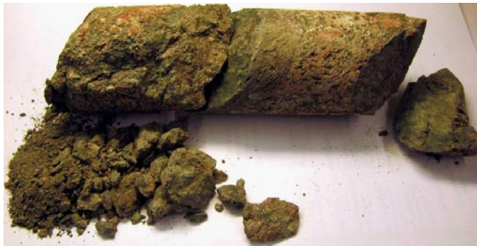
Photograph of the drill core KLX13A: 557.964–558.114 m characterised by highly fractured rock (cataclasite dominated) with high amount of fine-grained (crush) material.
