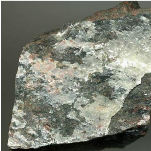
Photograph of the fracture surface of sample KLX13A: 506.750–506.999 m, consisting of calcite (bright) on top of e.g. chlorite.
