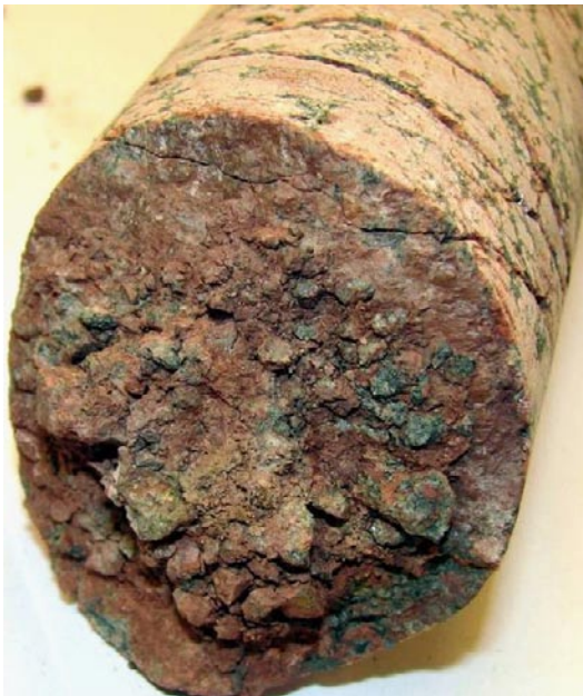
Photograph of drill core KLX17A: 110.274–110.544 m, showing a very rough fracture surface with variable thickness of the coating.
