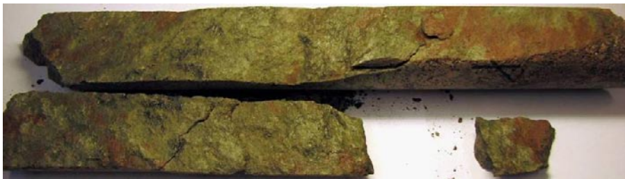
Photograph of the drill core KLX13A: 570.000–570.329 m, with smooth fracture surfaces dominated by clay minerals/chlorite along with hematite (red-stained parts) and wall rock fragments.
