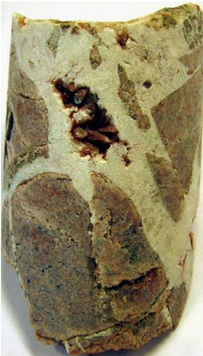
Photograph of sample KLX14A: 80.940–81.040 m, showing fractures sealed by mainly calcite. Cavities are partly filled with scalenohedral calcite coated by small amounts of hematite.
