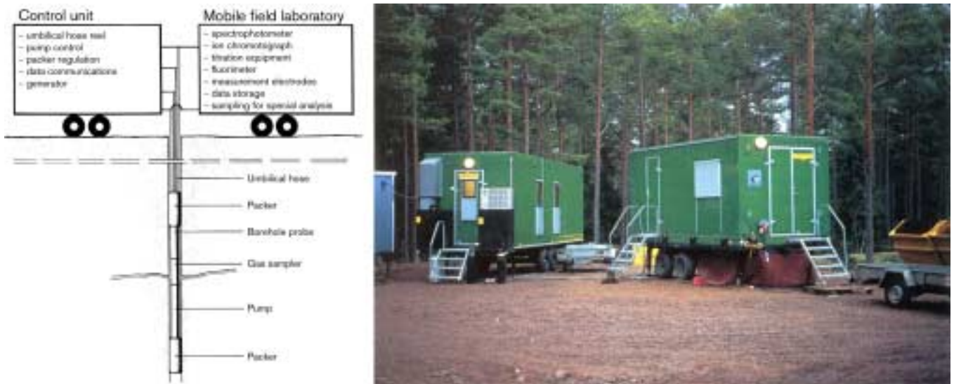
Figure 4-5. SKB's mobile hydrochemical sampling and analysis system.
