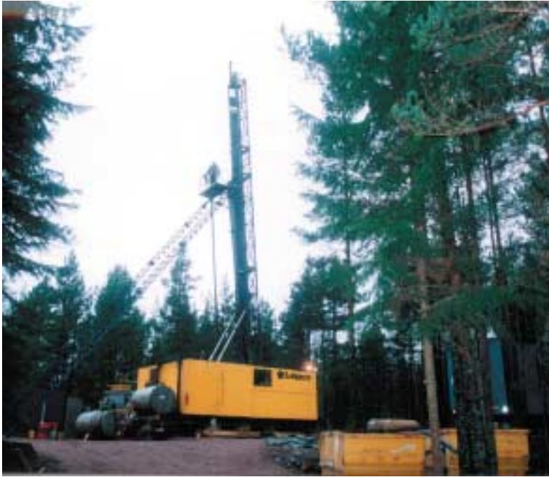
Figure 2-1. Core drilling on a prepared drilling site served by a road.
