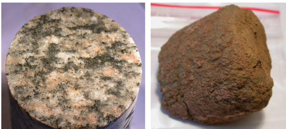
Figure 3-1. Pictures of rock samples selected for; a) electrical resistivity experiments (KFM02A 781.01 mbl (metres borehole length)), and b) batch sorption measurements (KFM06B 56.26 mbl).
