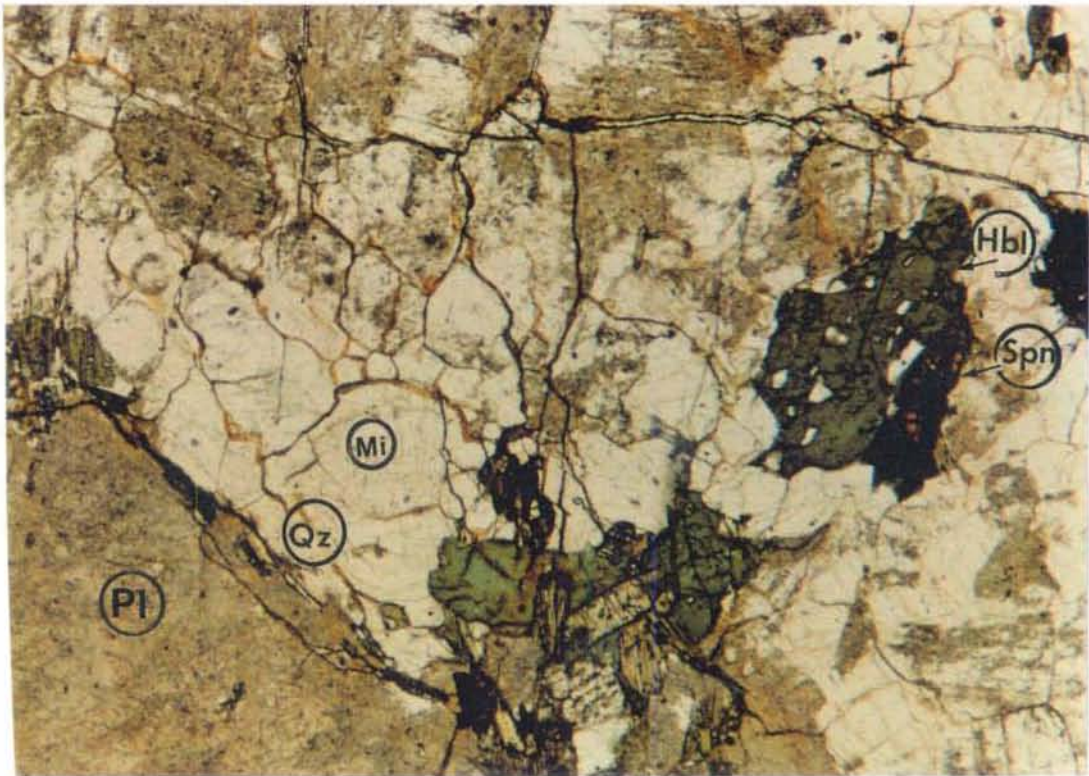
PLATE 1. Microphotograph of sample 1:15 illustrating the staining and sericitic alteration of plagioclase. Note the unaltered appearance of microcline and quartz. View about 3.5 mm. Plane-polarized light.
