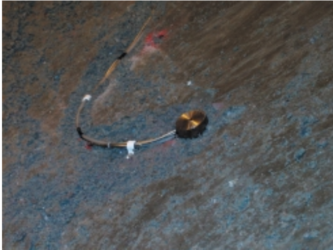
Figure 6-47. DPP sensor installed perpendicular to layer.
