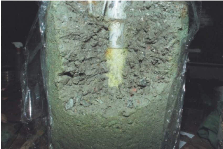
Figure 6-60. Detail of the sensor surrounded by the backfill after 15 months into the cell.
