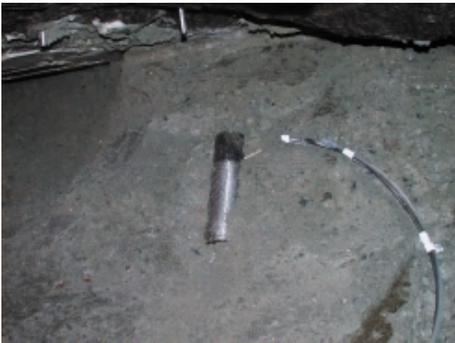
Figure 6-48. DPP sensor installed parallel to layer.
