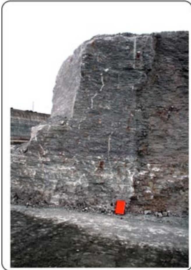
Figure 3-41. Large fault plane with very pronounced slickensides and striations. The plane strikes N-S and is a sinistral fault. View to 090°.
