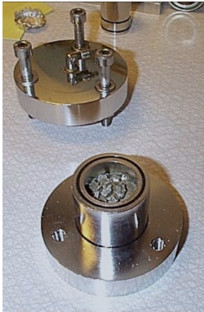
Figure 5-1. Typical appearance of the vapor-treated samples with crumbled upper part.
