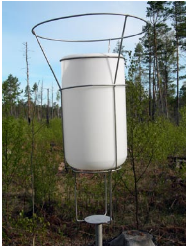
Figure 4-3. Precipitation sampler, winter setup. Two sampler setups were used simultaneously in order to increase the collected volume of the precipitation.
