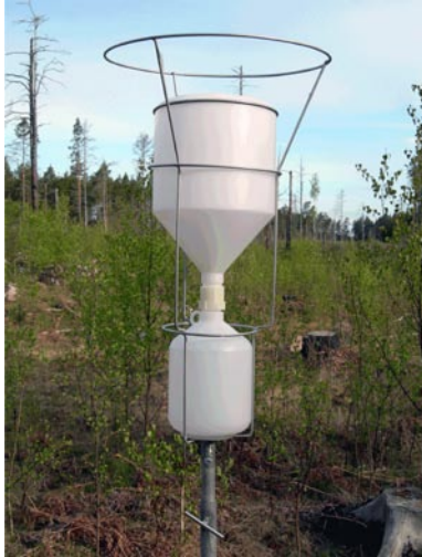
Figure 4-2. Precipitation sampler, summer setup. Two sampler setups were used simultaneously in order to increase the collected volume of the precipitation.
