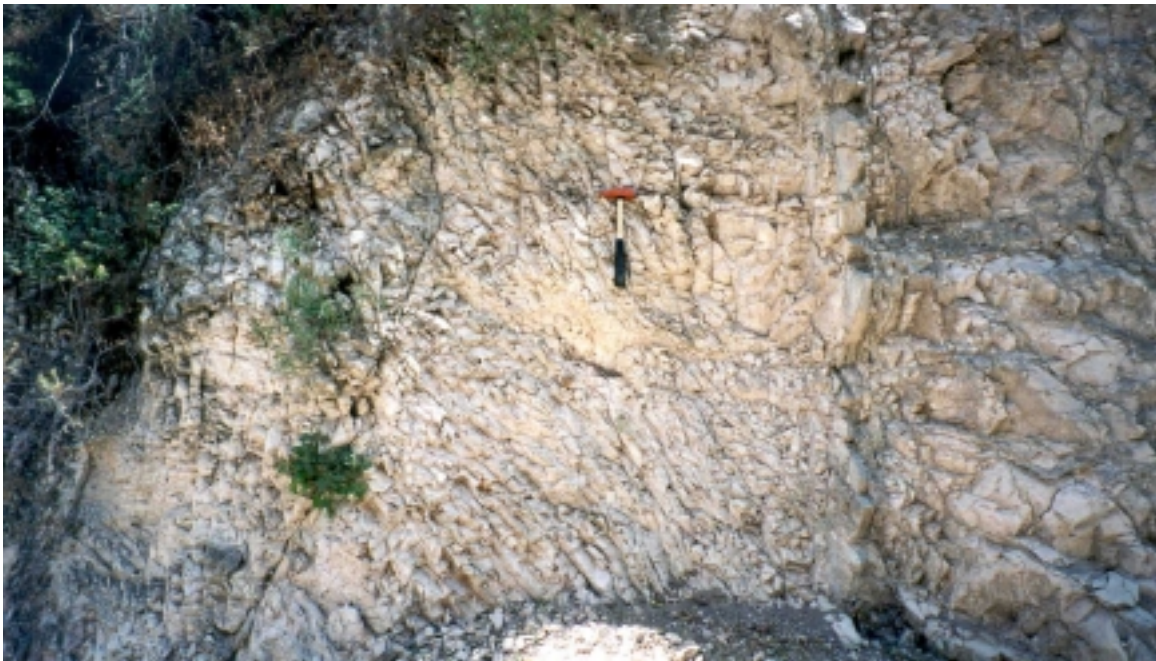
Figure 2-4. Zone of intense fracturing delineated from less fractured rock to the right by a thick calcite filled crack-seal vein.
