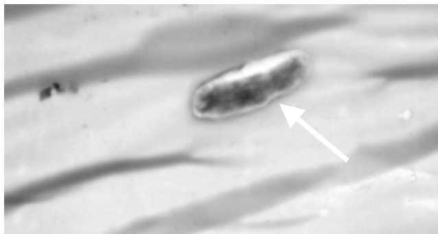
Figure 3-16. Transmission electron microscopy images of fracture material with bacterium-shaped structures (arrow) from BAX08, 10.70 m in the reactor (scale 1 cm = 0.5 \mu\text{m} ).
