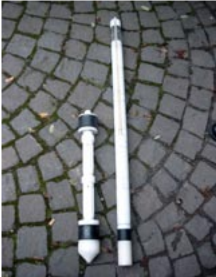
Figure 4-1. Double packer piston pump. On the left, the double packer with the two collars, which were pumped up with compressed air to define the stratum where the sample has to be pumped from. Right side: the piston pump unit. Photo: D. Matzke.
