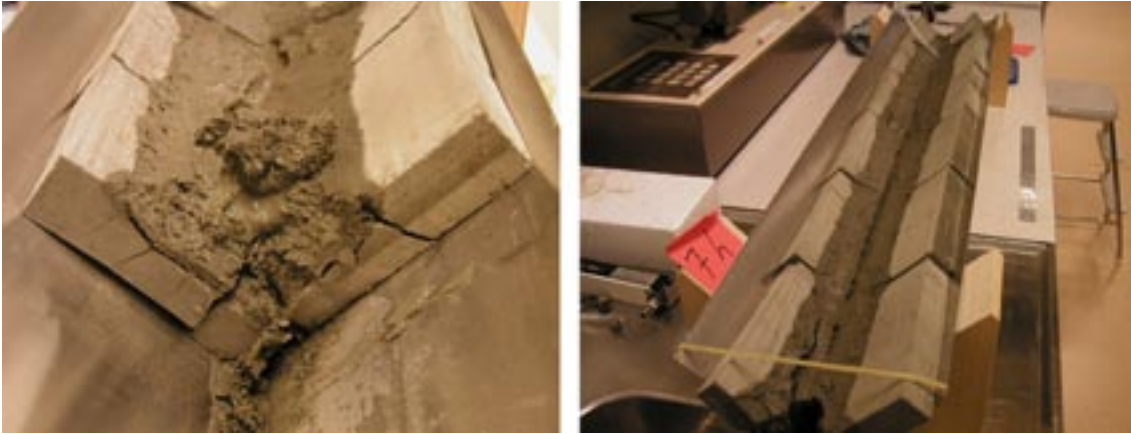
Figure A6-3. Pictures from the test. The left picture shows a section during the excavation. The right picture shows the situation just before the interruption. The surrounding block surfaces are strongly influenced of the water.
