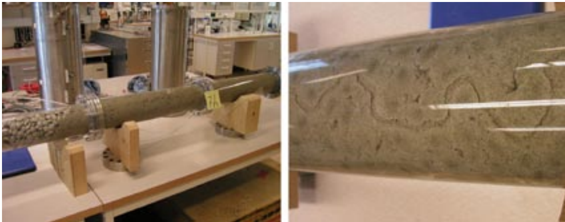
Figure A15-4. Pictures from the test. The left picture shows the situation after 7 hours during the water filling. The right picture shows the channel where all water seems to flow. The channel is situated on the top of the sample.
