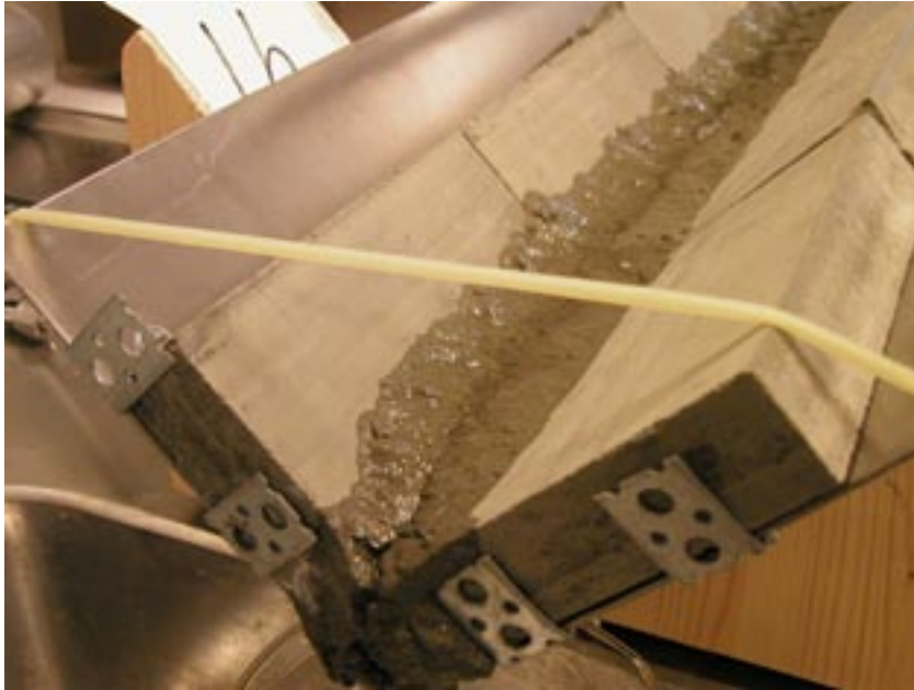
Figure 3-2. Picture showing a part of the used test equipment. In the front the steel angle-irons, locking the bentonite blocks, can be seen.
