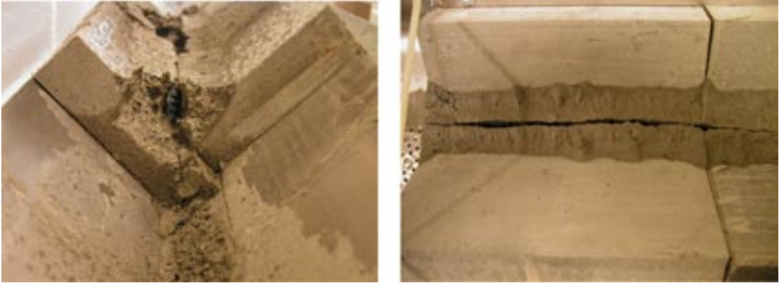
Figure A7-2. Pictures from the test. The left picture shows a section during the excavation. The right picture shows the situation just before the interruption. There was a sharp ditch in the middle.
