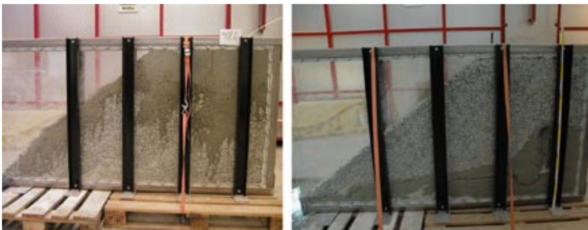
Figure 7-1. Pictures from the slot tests. The picture to the left shows the test where a water flow rate of 0.01 l/min was applied and the picture to the right the test with a water flow rate of 1 l/min.
