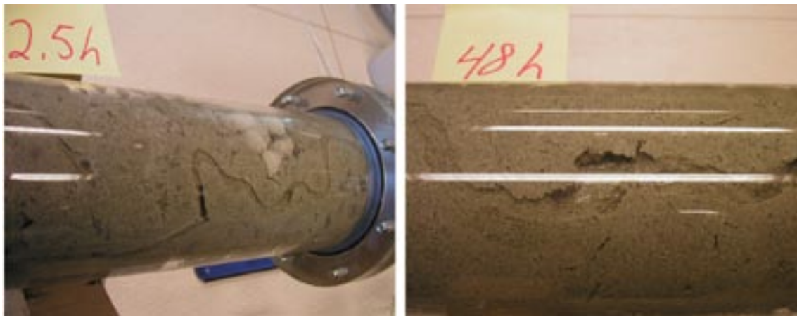
Figure A16-4. Pictures from the test. The left picture shows the situation after 2.5 hours during the water filling. The right picture shows the channel were all water seems to flow. The channel is situated on the top of the sample.
