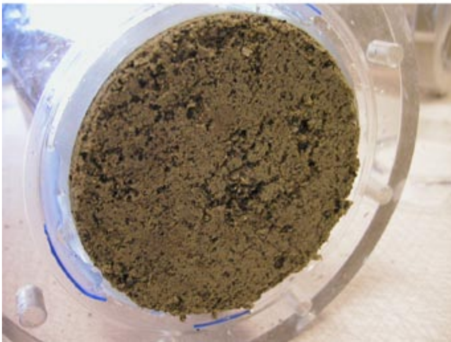
Figure A19-3. Pictures from the test. The upper picture shows the situation after 40 minutes during the water filling. There is a very clear front of the water. The right picture shows the inlet side at dismantling. The material is quite loose here. No special channel can be detected. The material seems to be very evenly wetted.
