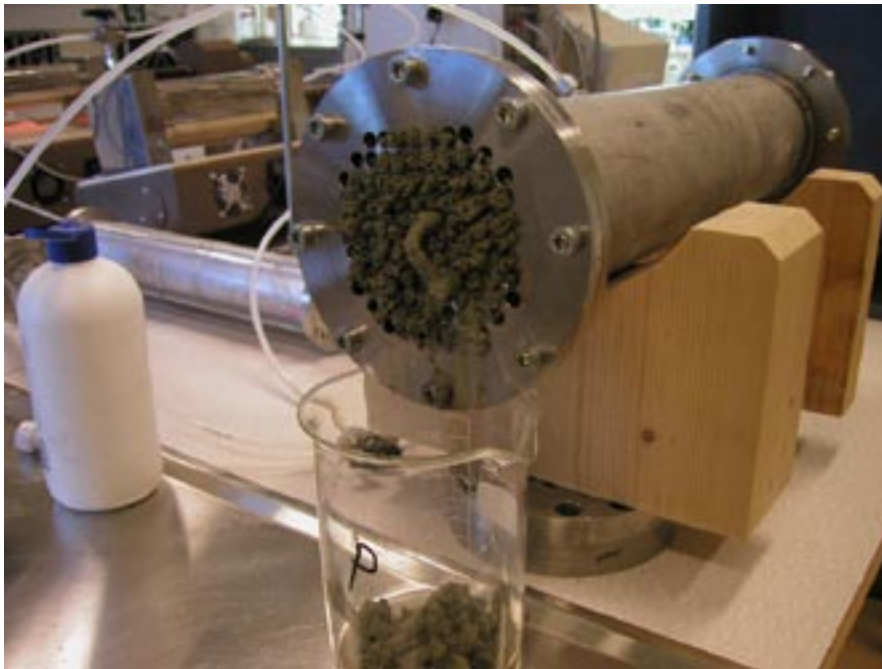
Figure A21-4. Picture from the test showing the situation when the higher flow has been applied and the pressure is rising. The material is pushed out in both ends of the sample holder.
