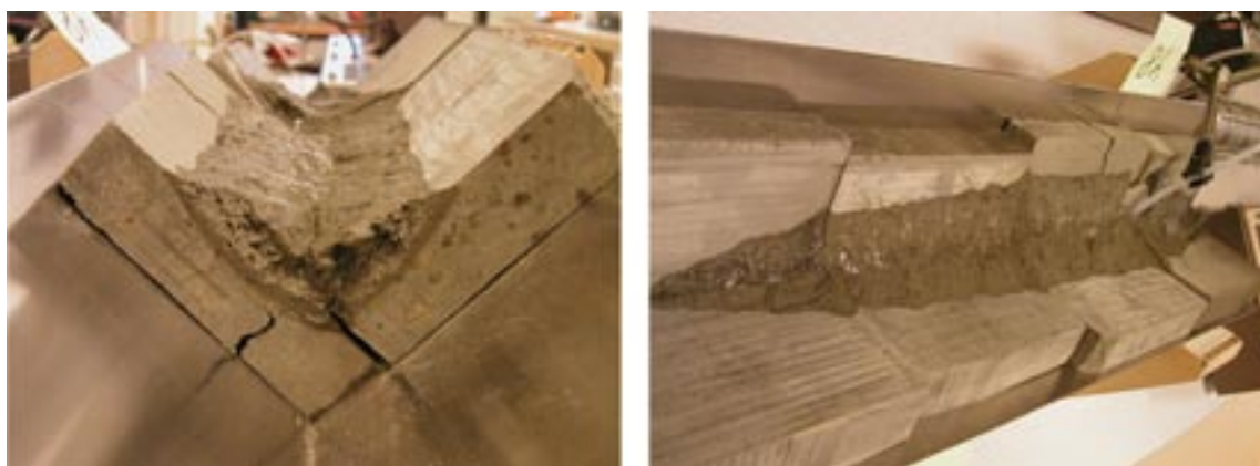
Figure A4-1. Pictures from the test. The left picture shows a section during excavation. The right picture shows the situation just before the interruption. Due to the low flow rate, no erosion took place.
