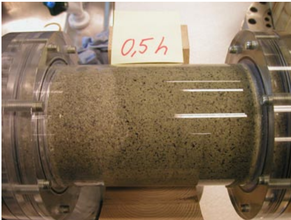
Figure A17-2. Picture from the test showing the situation after 0.5 hour. There is a very clear front of water saturation.
