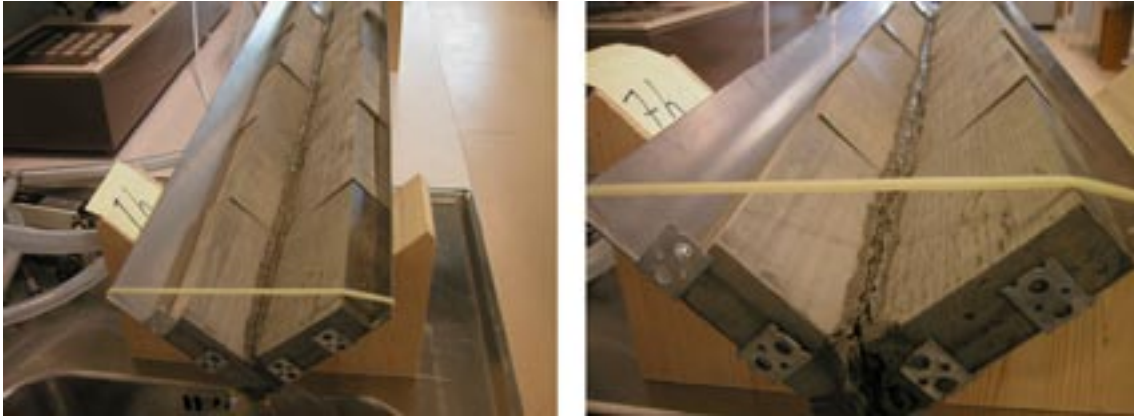
Figure A1-3. Pictures from the test. The picture to the left shows the situation after one hour. The right picture shows the situation just before the interruption. There is a small sharp ditch in the middle. The surrounding block surfaces are not affected.
