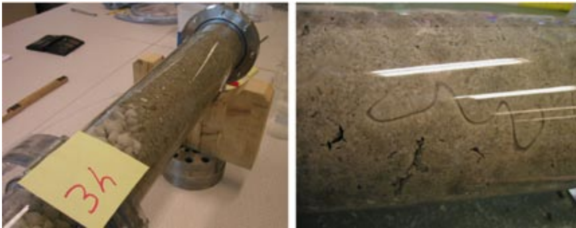
Figure A9-4. Pictures from the test. The left picture shows the situation after 3 hours during the water filling. The right picture shows the channel where all water seems to flow. The channel is located on the top of the sample.
