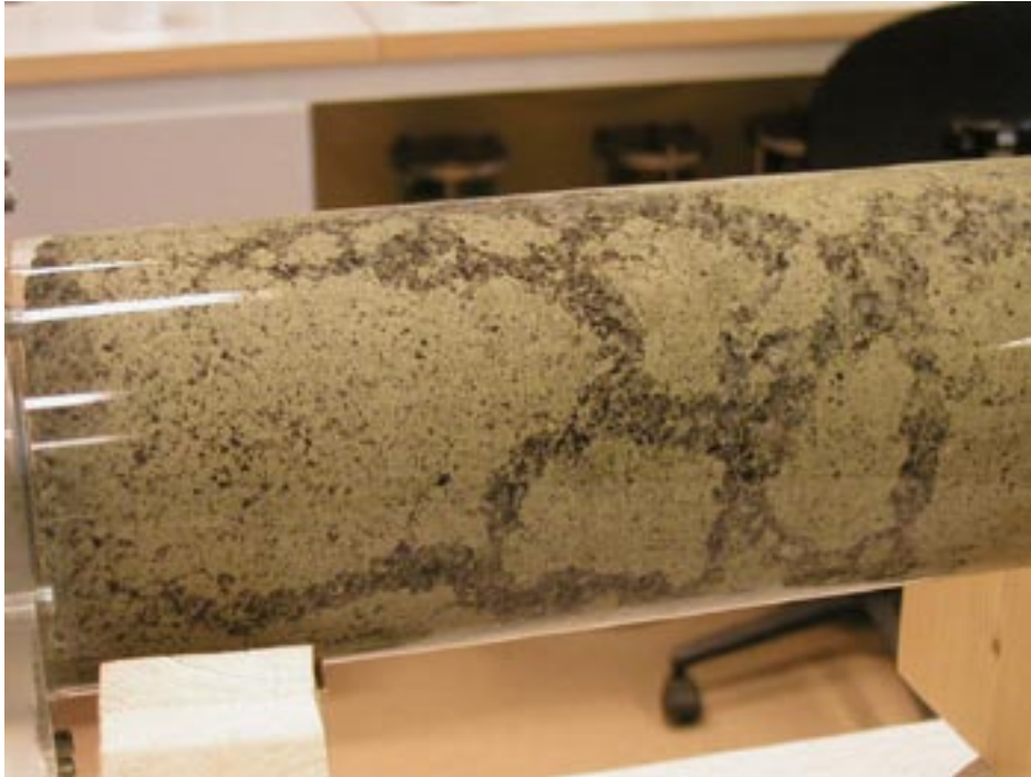
Figure A20-3. Picture showing the outer surface of the sample. At first the wetting was done as a front, but the water was after a few minutes located to channels. In the channels the bentonite was washed out leaving the crushed rock left. In spite of the channels, the pressure was raised to about 1,400 kPa and the test had to be interrupted.
