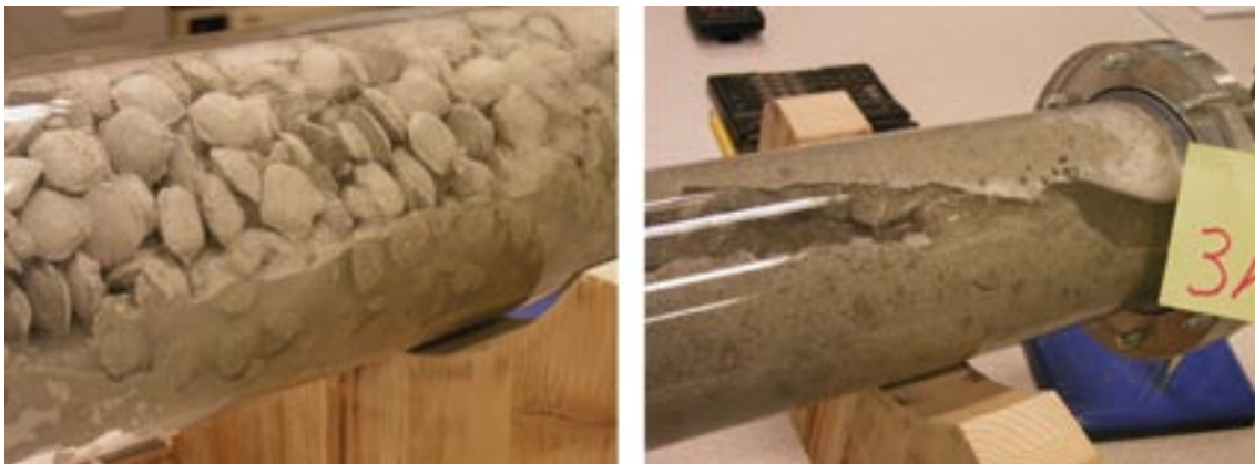
Figure A14-4. Pictures from the test. The left picture shows the situation after 3 hours during the water filling. The right picture shows the channel where all water seems to flow. The channel is situated on the top of the sample.
