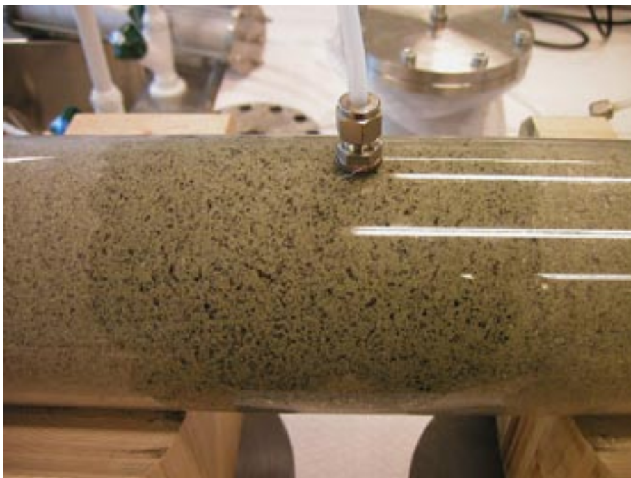
Figure A22-2. Picture showing the water inlet positioned on the middle of the tube.
