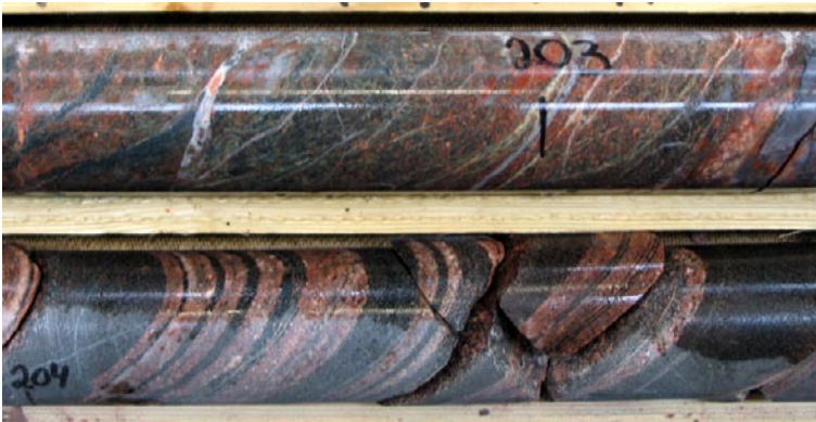
Figure 5-38. Close-up of drill core at ca 203 m showing different types of sealed fractures and cataclasites. Thin, chlorite- and epidote-sealed shear zones and fractures are cut by thin veins sealed with calcite and laumontite (for details, see Figure 5-39).
