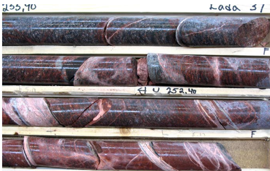
Figure 5-45. Example of drill core from DZ2 of KFM12A (ca 252–254 m). Faults sealed with laumontite and calcite are present. In general, these brittle structures post-date fractures coated and/or sealed with chlorite, clay minerals and hematite.
