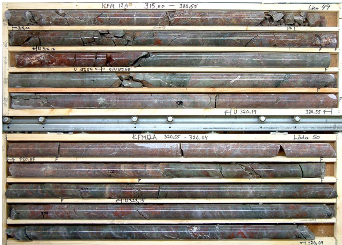
Figure 5-51. Photograph showing drill core from DZ2 at ca 315–326 m. The drill core consists of greenish, reddish and grey proto-cataclasite, cataclasite and fault breccia. Minor ultra-cataclasite occurs in up to 20 mm wide zones.
