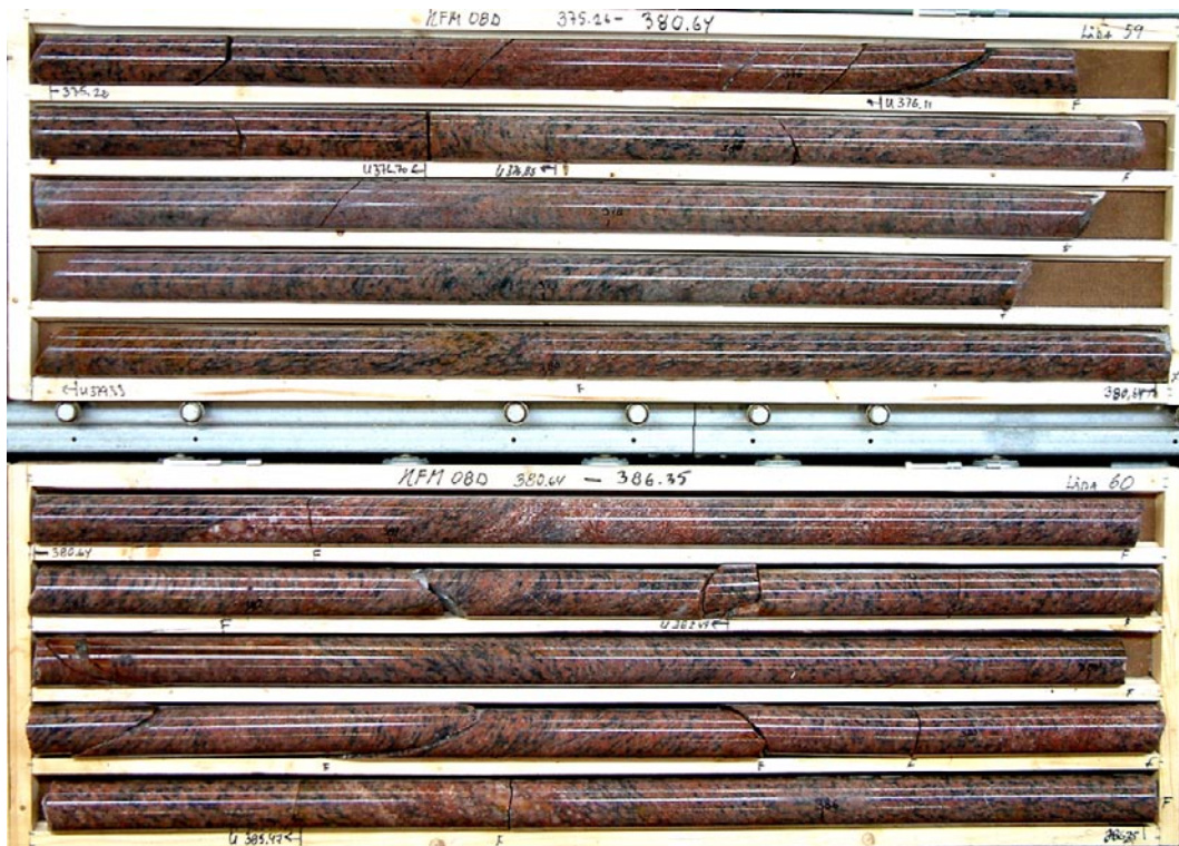
Figure 5-16. Photo showing weakly oxidized metagranite-granodiorite with some pegmatite from the central part of DZ3. Brittle deformation products are mainly represented by some sealed fractures.
