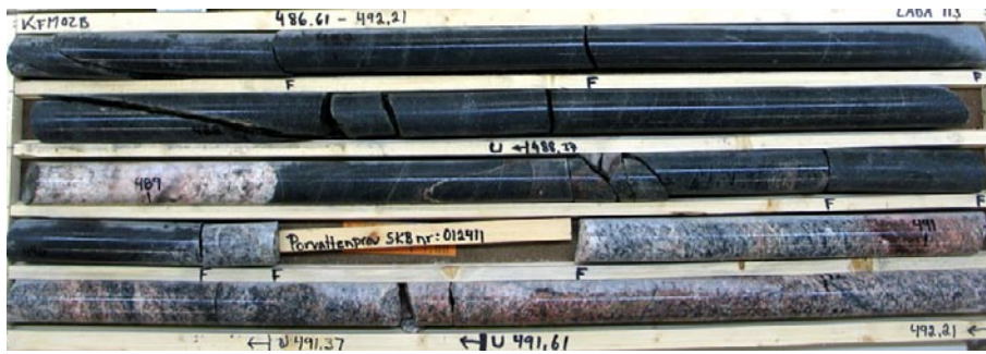
Figure 5-12. Photograph of drill core from the uppermost part of DZ6 of KFM02B (486.6–491.6 m). Steep fractures with epidote and some chlorite and gently dipping epidote-sealed thin fractures are present in the amphibolite.
