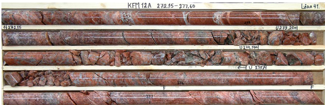
Figure 5-47. Photograph showing oxidized pegmatite and metagranite from DZ2. A significant crush zone forming a fault core is present at 274–275.5 m. The fractures are coated with chlorite and clay minerals.
