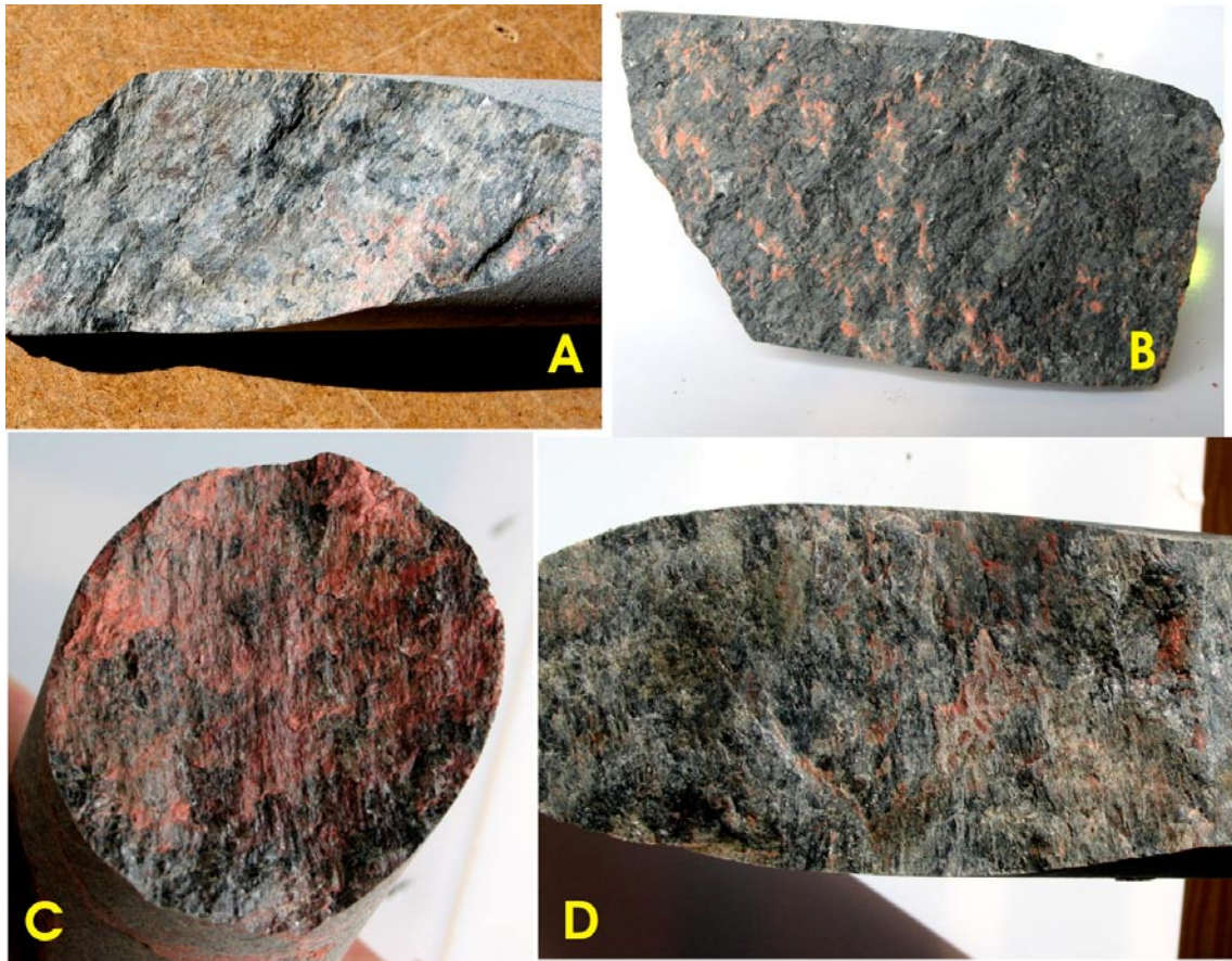
Figure 5-31. Photographs illustrating fault surfaces observed in DZ1 of KFM11A. A: reverse fault surface (518.59 m, strike/dip and pitch: 53/78–74) with slickensides and steps defined by chlorite, hematite and clay minerals. B: reverse fault surface (525.60 m, strike/dip and pitch: 305/76–42) with chlorite slickensides and laumontite steps. C: normal fault surface (525.95 m, strike/dip and pitch: 135/78–77) with slickensides and steps with chlorite and laumontite. D: reverse fault surface (571.14 m, strike/dip and pitch: 17/52–86) with slickensides and steps defined by chlorite, laumontite and clay minerals.
