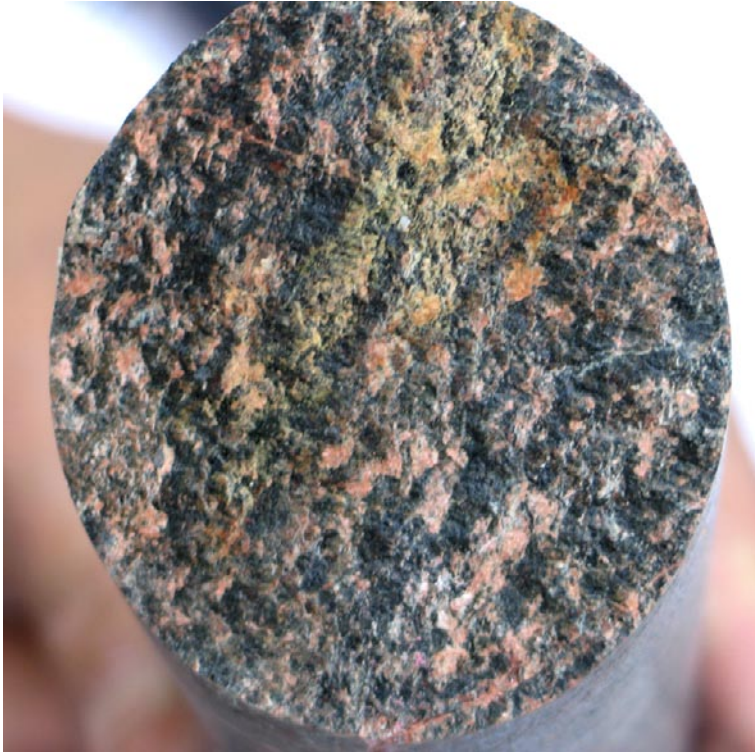
Figure 5-46. Photograph illustrating fault surface observed in DZ2 of KFM12A. Chlorite striation and steps with laumontite provides kinematic data (253.78 m, strike/dip and pitch: 132/85–72).
