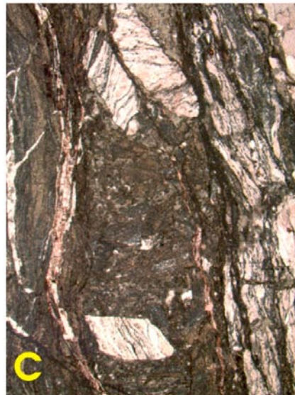
Figure 5-40. Scanned thin section (A) and photomicrographs (B and C) of sample KFM12A_204.9. The thin section (width of view is 38 mm) shows foliated metagranite cut by dark greenish, foliated shear zone rich in chlorite (right). The metagranite adjacent to the shear zone has a mylonitic texture. The shear zone has been reactivated and the central part is a fine-grained ultra-cataclasite with angular fragments of the mylonite (C). The cataclasite shown in B is chlorite-rich with angular fragments of the metagranite. The metagranite between the shear zone/cataclasites is riddled with thin fractures with minor development of cataclasite.
