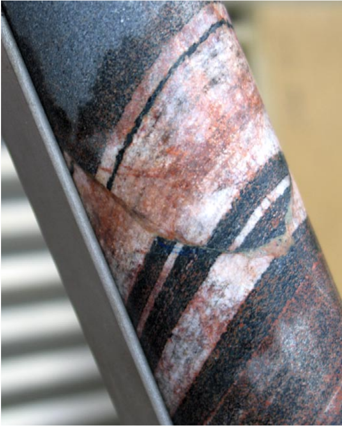
Figure 5-37. Close-up of drill core showing a small fault that cuts lithological boundaries at ca 192.5 m. The normal fault has dip slip movement and is oriented 358/39.
