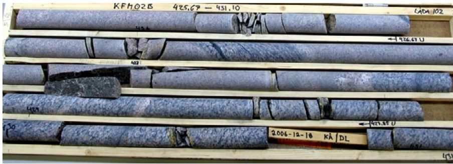
Figure 5-7. Example of drill core from the lower part of DZ3 of KFM02B (425.5–431 m). Note the presence of gently-dipping un-mineralized fractures and some steep fractures with chlorite and minor calcite.
