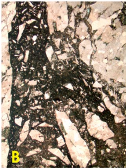
Figure 5-40. Scanned thin section (A) and photomicrographs (B and C) of sample KFM12A_204.9. The thin section (width of view is 38 mm) shows foliated metagranite cut by dark greenish, foliated shear zone rich in chlorite (right). The metagranite adjacent to the shear zone has a mylonitic texture. The shear zone has been reactivated and the central part is a fine-grained ultra-cataclasite with angular fragments of the mylonite (C). The cataclasite shown in B is chlorite-rich with angular fragments of the metagranite. The metagranite between the shear zone/cataclasites is riddled with thin fractures with minor development of cataclasite.
