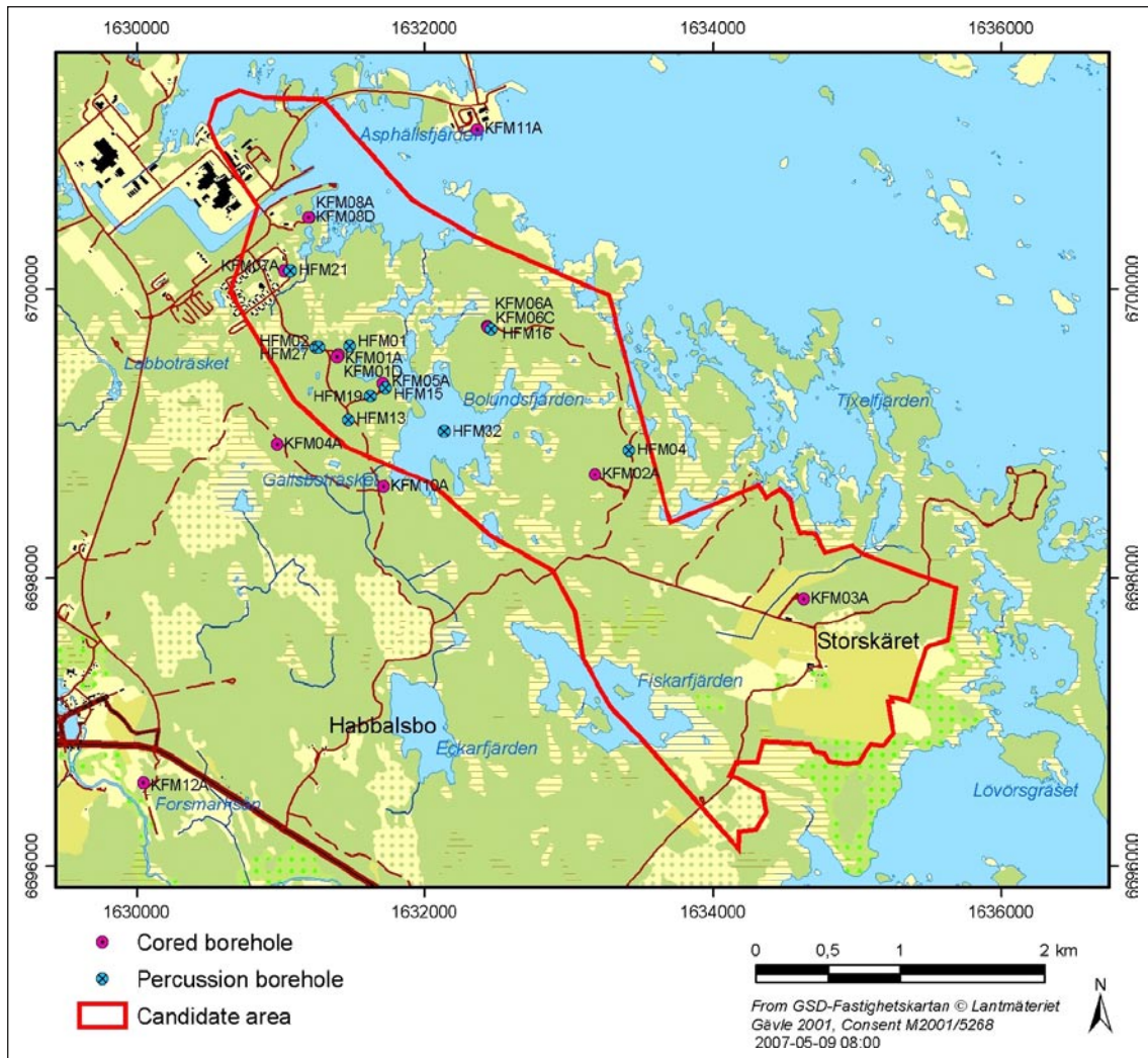
Figure 1-1. Overview over Forsmark site investigation area, showing locations of boreholes included in this activity.
